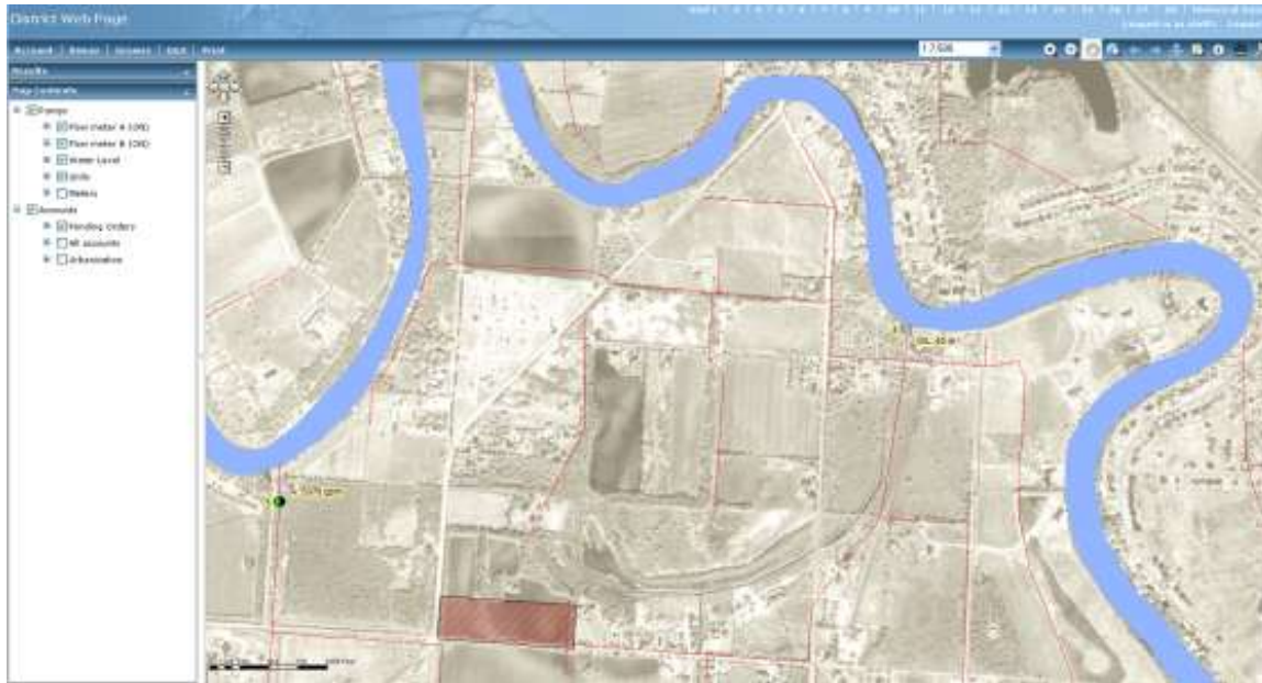
Figure 10. Aerial photographs are combined in a single layer and cached using the ArcGIS Image Server extension
