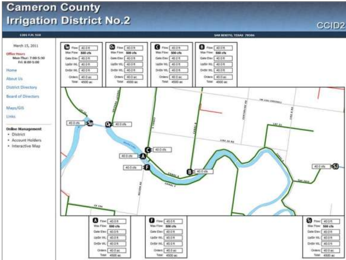
Figure 9. Status map set for CCID2, which displays information for the automated Rubicon gates in the Warley Lake resaca area (demonstration only).
