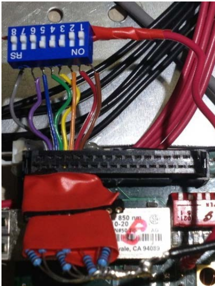
Figure 9: GEM pad ID selection switches, which attach to the table-top TMB. The blue device allows the user to input a GEM pad ID number in binary.
