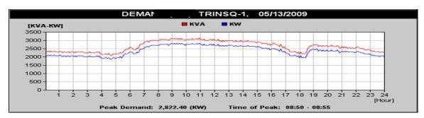
RTM allows the monitoring of energy consumption in 5 minute increments. Alarms notify operators when the use, demand, price exceeds a predetermined limit. Operators are now empowered to take action, such as shift a portion of the load during price spikes so that energy savings and / or demand savings can be realized.
