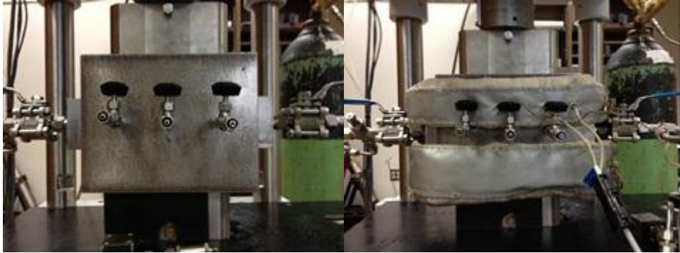
Fig 2.12: Final Assembly of the Conductivity Cell
