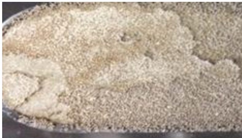
Fig 3.1: Proppant Cake Formed at High Temperature Experiments
