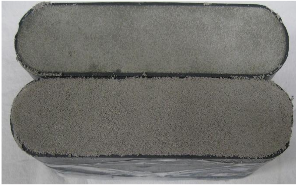
Fig 3.5 Experiment with Uniform Proppant Distribution
