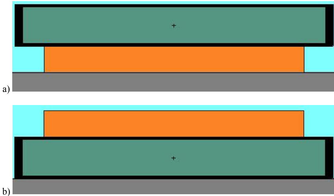
Fig. 5.5. Calibration source geometry with source a) between and b) opposite the concrete background source.
