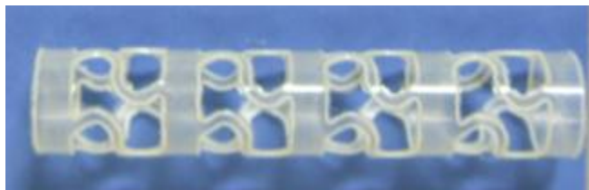
Figure 36 – Prototype of a shape memory polymer neurovascular stent. Courtesy of Landon Nash, Texas A&M University.
