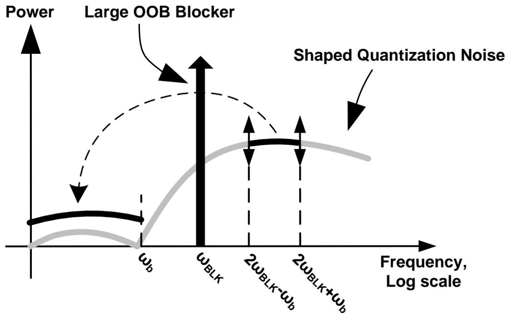
**Fig. 7.2. Noise folding caused by intermodulation between OOB blocker and shaped quantization noise.**
