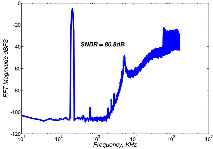
**Fig. 2.18. PSD at the modulator output calculated using 32768 FFT points with 16 averages. Signal Amplitude =  $-4$  dBFS, Signal Frequency = 270 KHz.**
