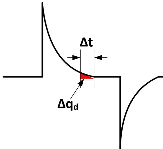
Fig. 2.6. Jitter-tolerant exponentially-decaying waveform.
