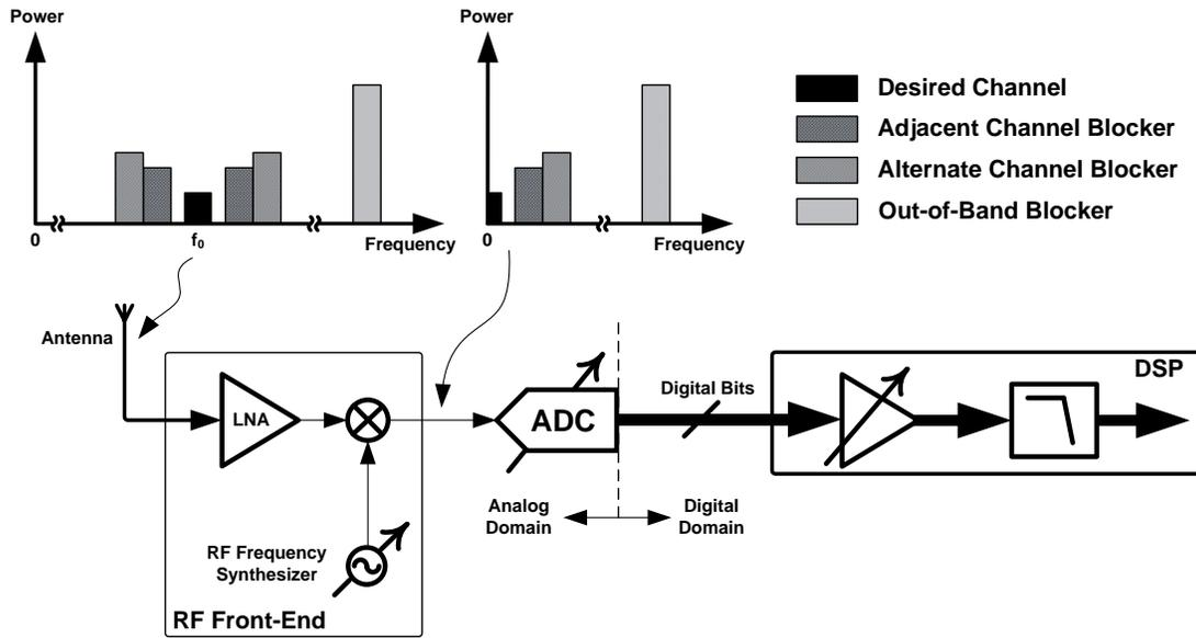
**Fig. 3.6. Candidate architecture for SAW-less multi-standard/multi-band and software-defined radio receivers.**
