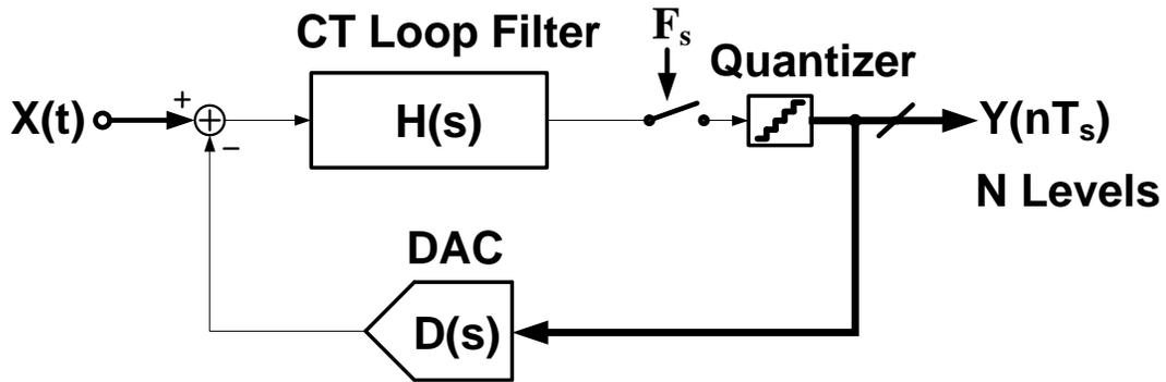
**Fig. 1.4. Continuous-time  $\Delta\Sigma$  modulator block-diagram.**
