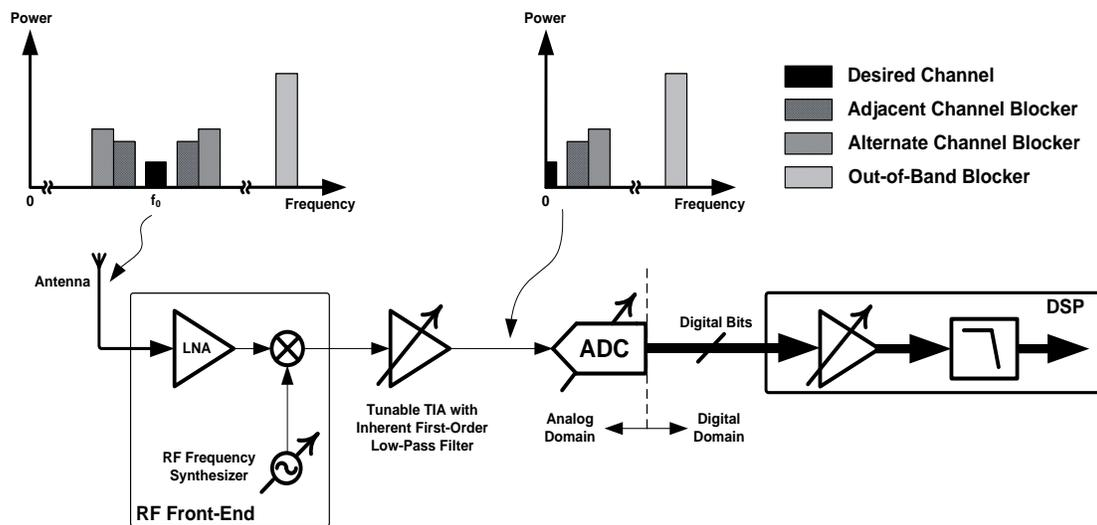
**Fig. 1.1. Candidate architecture for SAW-less multi-standard/multi-band and software-defined radio receivers.**
