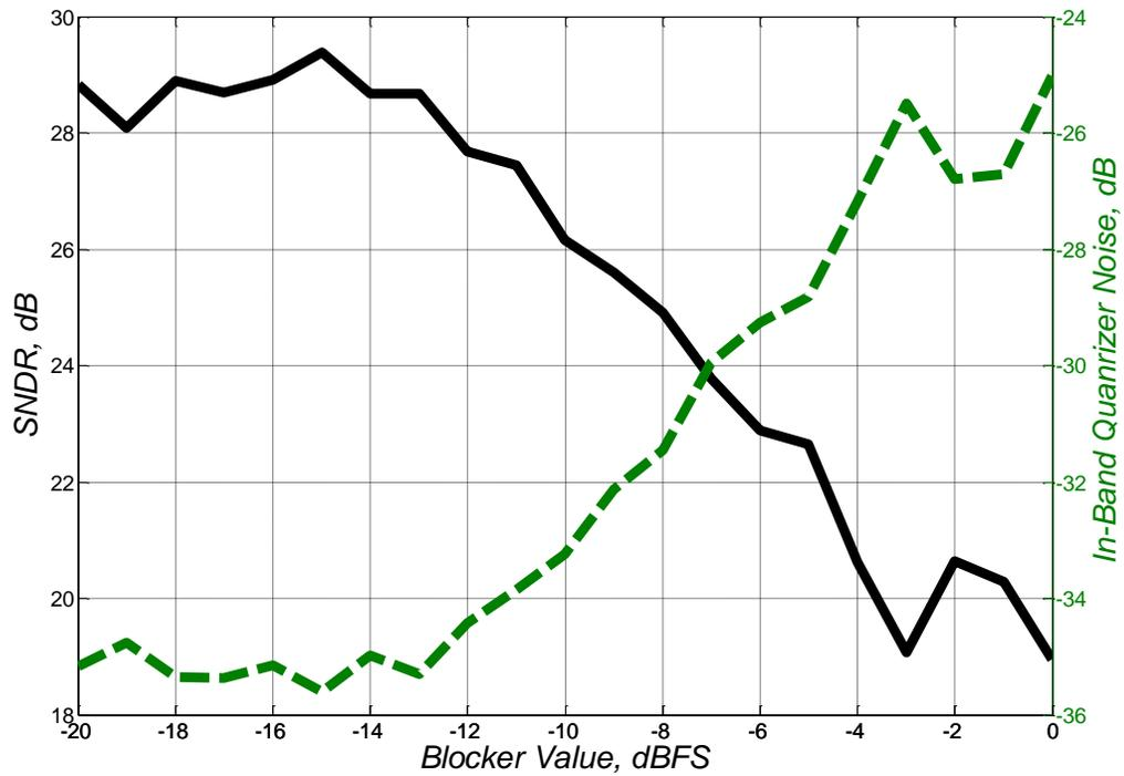
**Fig. 4.3. Variation of the SNDR and the in-band quantizer noise power with the input blocker.**
