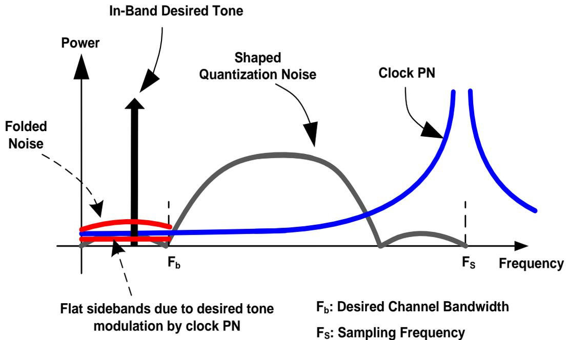
**Fig. 2.11. Modulation of in-band desired signal and shaped quantization noise by phase-noise in the DAC sampling clock.**
