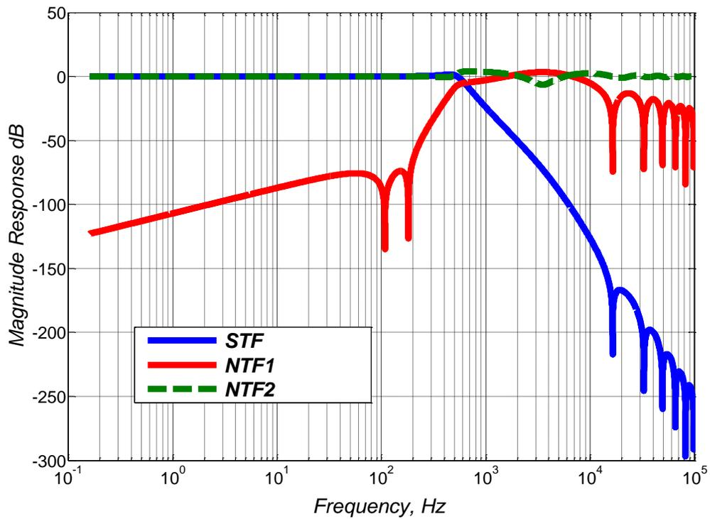
**Fig. 4.2.** Magnitude responses for signal and noise transfer functions at quantizer input and output terminals for the  $\Delta\Sigma$  modulator in Fig. 4.1.
