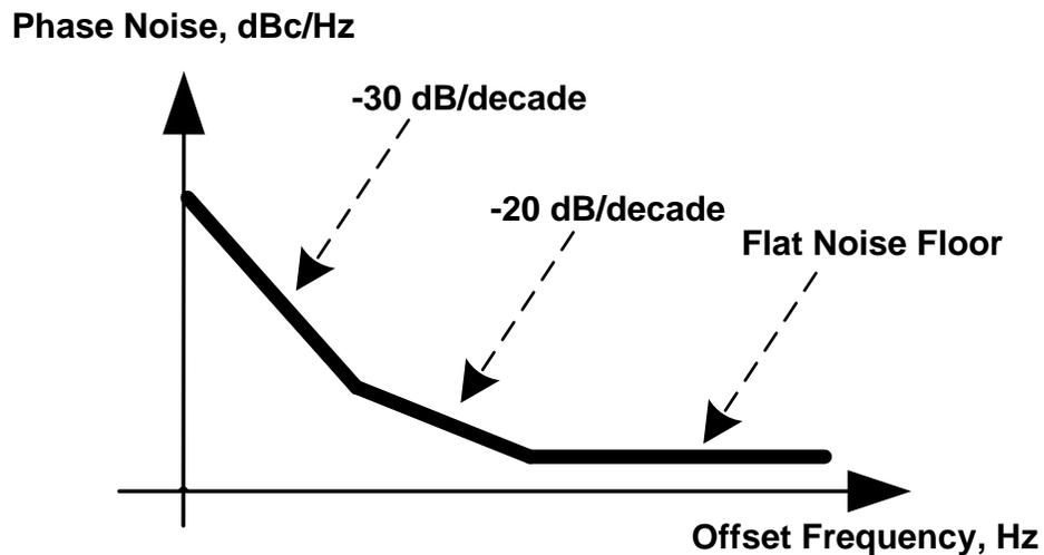
**Fig. 2.1. Typical phase-noise profile in a VCO.**
