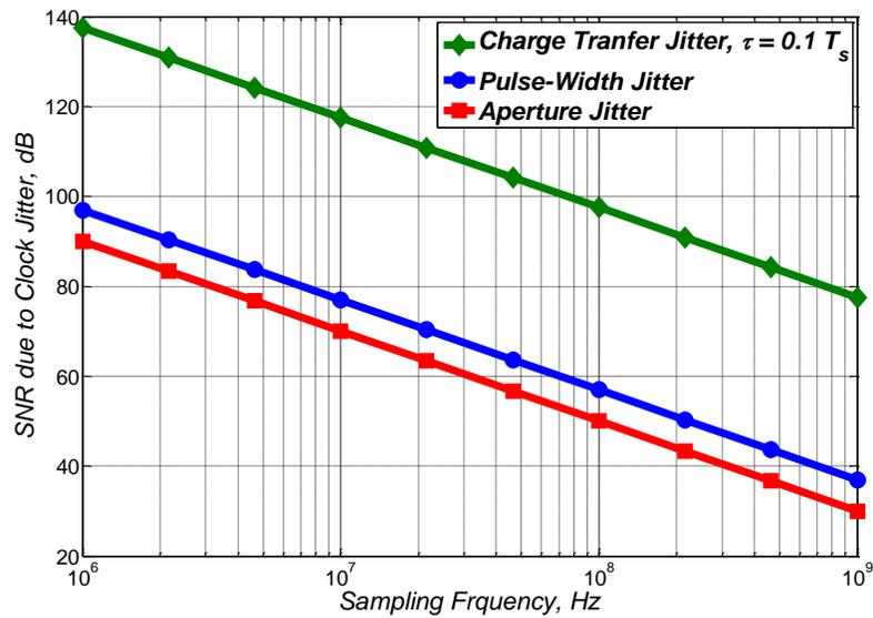
Fig. 2.9. SNR variation with the sampling frequency due to different types of jitter induced errors for a rms jitter of 10 ps.
