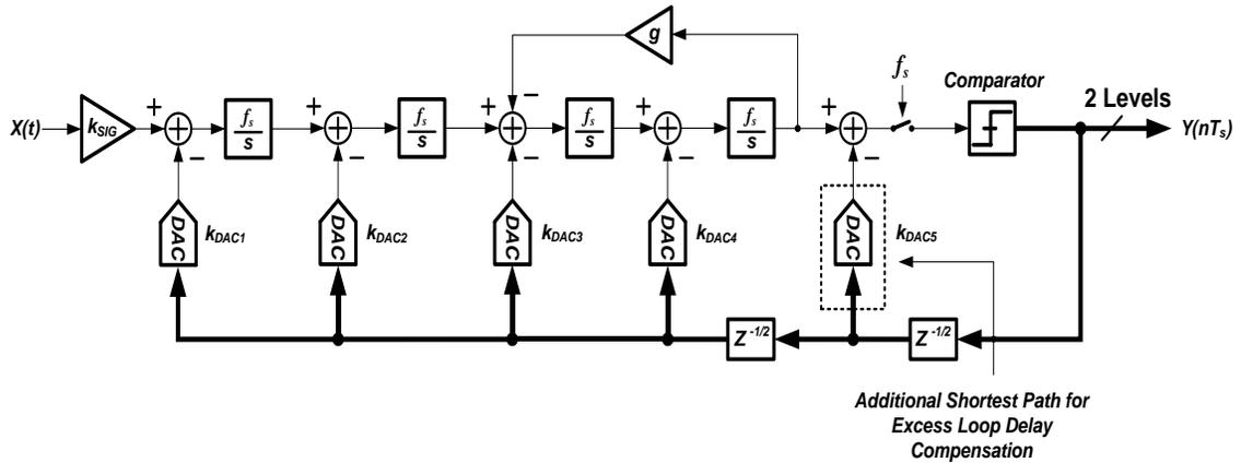
**Fig. 6.3. Fourth-order single-bit continuous-time  $\Delta\Sigma$  modulator in cascade-of-resonators-feedback (CRFB) structure.**
