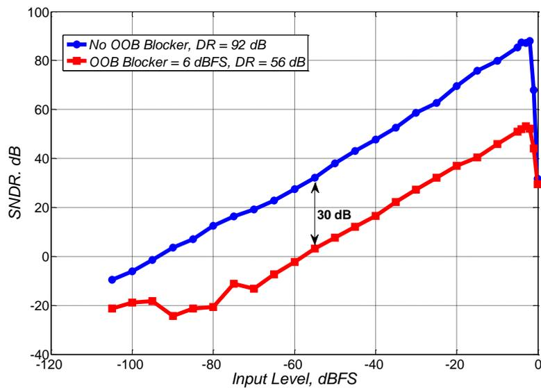
**Fig. 7.5.** DR degradation due to noise folding in presence of a 6 dBFS OOB blocker tone at 5.6 MHz,  $f_{SIG} = 31$  KHz, first stage  $IIP_3 = 23$  dBFS.
