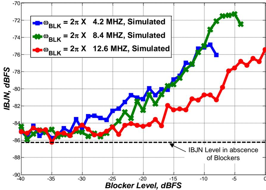
**Fig. 5.4.** Sensitivity of a feedforward 6-level third-order CT  $\Delta\Sigma$  modulator with NRZ DAC waveform to OOB blocker levels at the modulator input, in terms of total IBJN.  $\omega_{BLK} = 2\pi \times 12.6\text{MHz}$ ,  $V_{SIG} = -75\text{dBFS}$ ,  $f_{SIG} = 31\text{KHz}$ ,  $\sigma_j = 0.1\% T_S$ .
