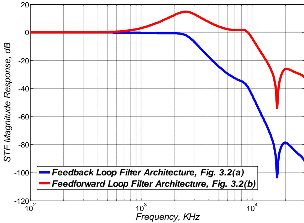
**Fig. 3.7.** STFs for the CT  $\Delta\Sigma$  modulators in Fig. 3.2.
