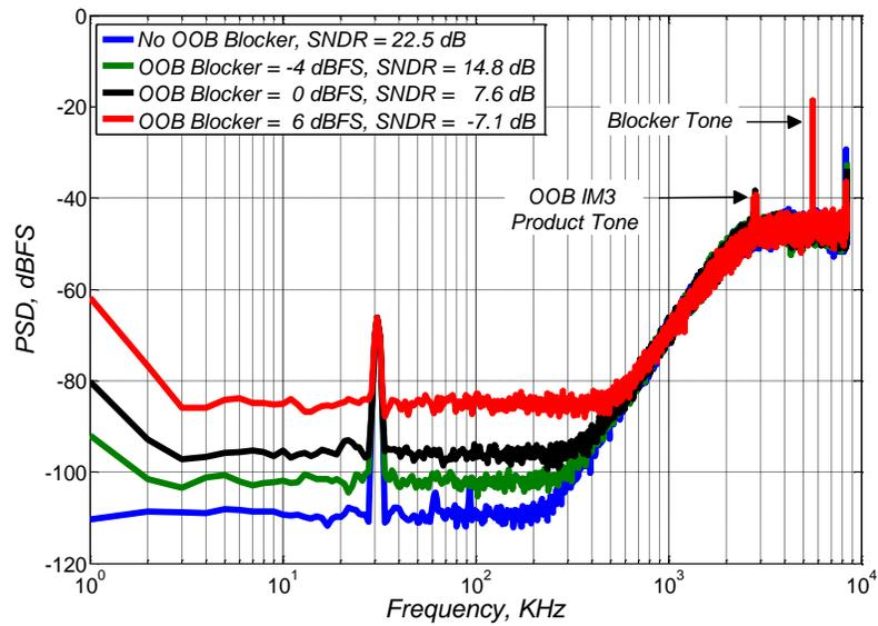
**Fig. 7.4.** Power spectra at the output of a third-order CT modulator in presence of an OOB blocker tone at 5.6 MHz,  $A_{SIG} = -65$  dBFS,  $f_{SIG} = 31$  KHz, first stage  $IIP_3 = 23$  dBFS.
