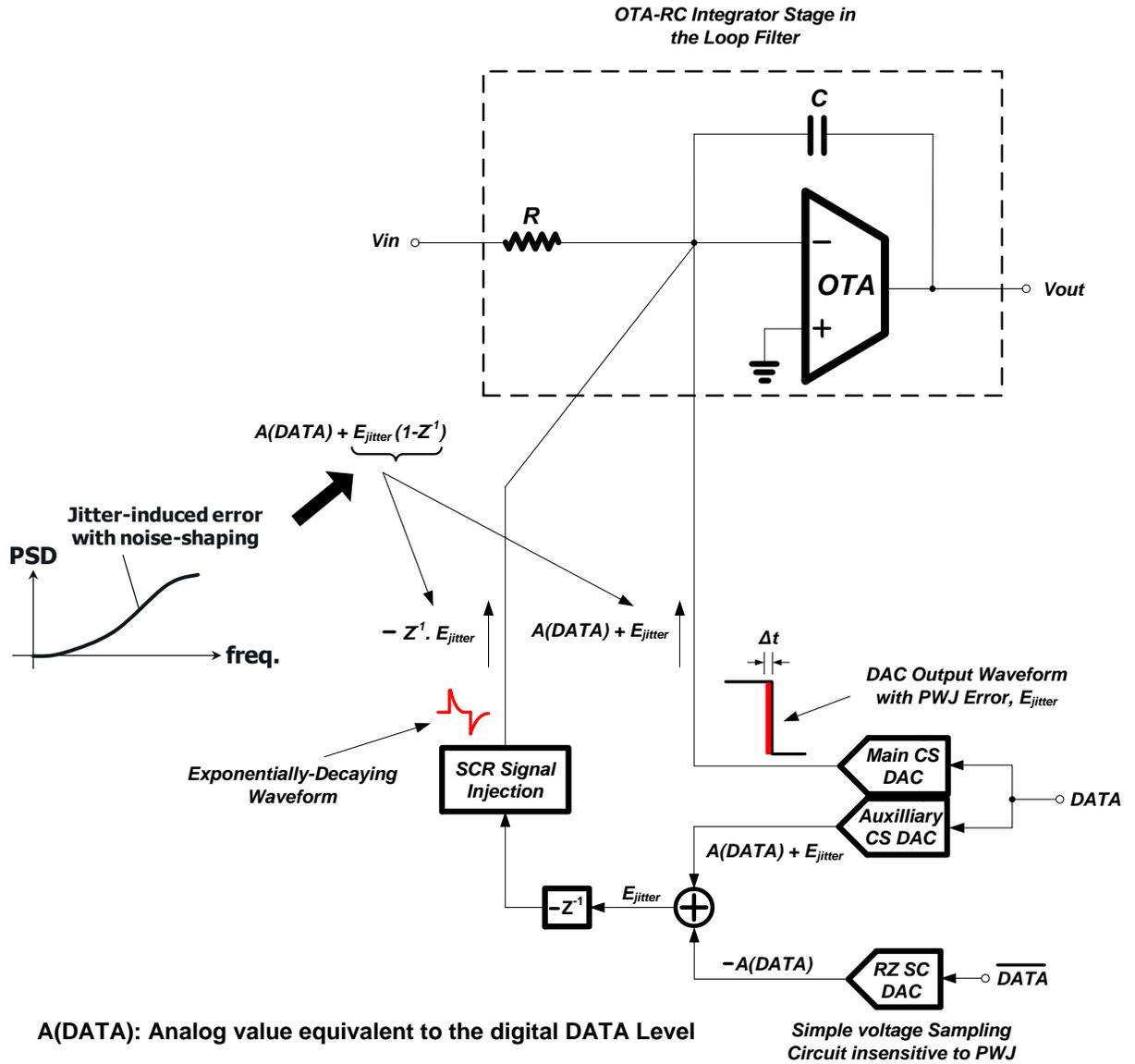
Fig. 6.2. Block-diagram for the proposed hybrid DAC solution based on spectral shaping of jitter induced errors.
