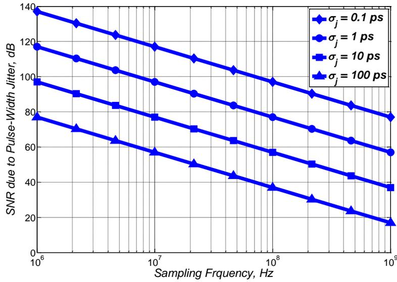
Fig. 2.8. SNR variation with the input frequency due to pulse-width jitter for different rms jitter values.
