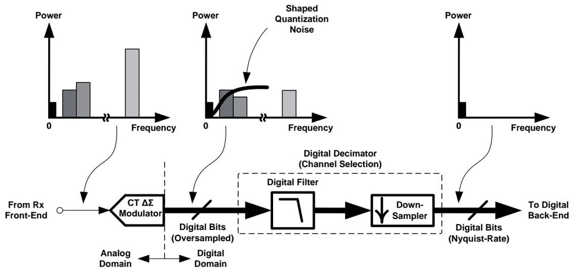
**Fig. 1.3. Continuous-time  $\Delta\Sigma$  ADC ( $\Delta\Sigma$  pulse density modulation + digital decimation and filtering), with inherent blocker filtering.**
