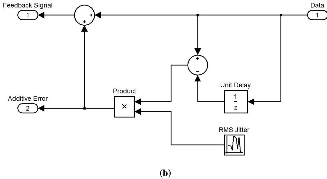
**Fig. 2.15. Simulink Modeling for DACs and jitter induced additive errors in the feedback of a CT  $\Delta\Sigma$  modulator. (a) RZ DAC. (b) NRZ DAC. (c) SCR DAC.**
