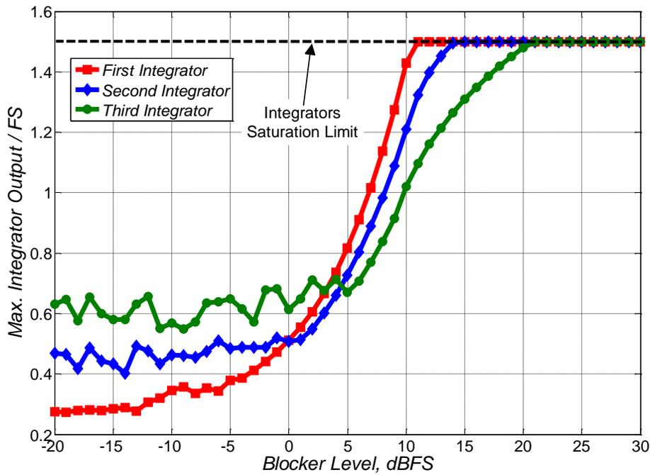
**Fig. 3.3.** Maximum integrator output swing variation with the OOB blocker level,  $f_{BLK} > f_u$ .
