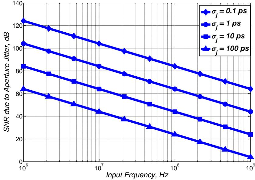
**Fig. 2.3. SNR variation with the input frequency due to aperture jitter for different rms jitter values.**
