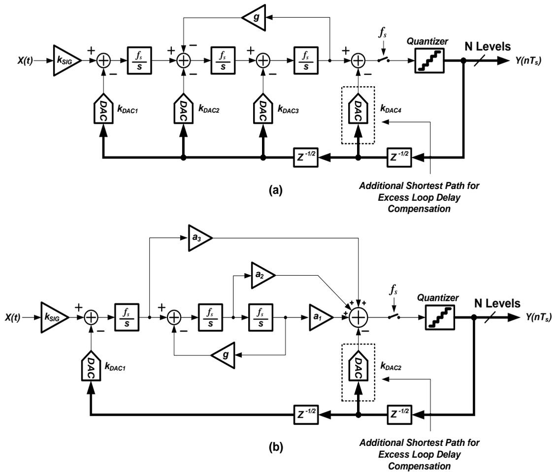
**Fig. 3.2. CT  $\Delta\Sigma$  modulators examples (third-order). (a) Feedback structure. (b) Feedforward structure.**
