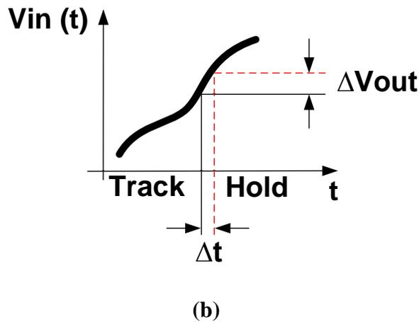
**Fig. 2.2. T/H Circuit. (a) Schematic view and clock waveform. (b) Effect of aperture jitter on sampled values.**
