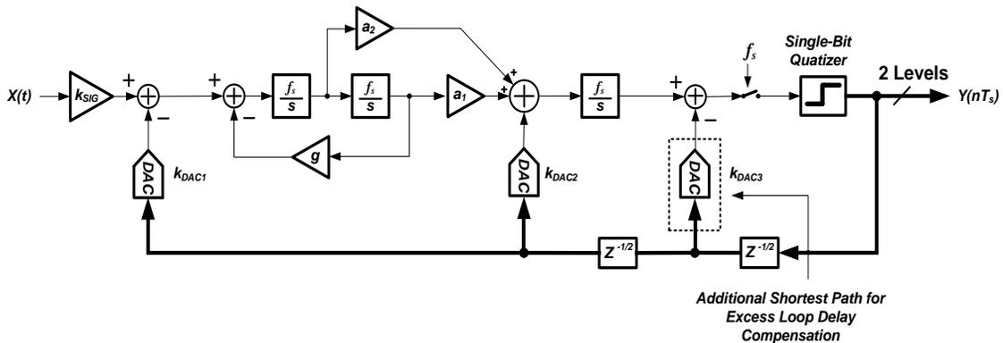
**Fig. 2.16. Adopted modified feedforward CT single-bit  $\Delta\Sigma$  modulator.**
