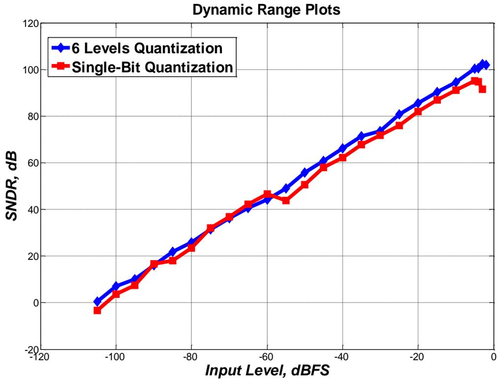
**Fig. 5.5. Dynamic-range plots for two equivalent feedforward third-order CT  $\Delta\Sigma$  modulators with 6-levels and single-bit quantization.**
