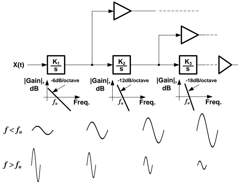
**Fig. 3.1. Magnitude responses of feedforward paths of loop filter to input sinusoids.**
