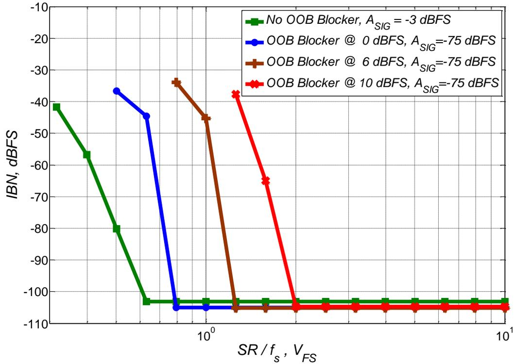
**Fig. 3.4. IBN of a third-order CT modulator due to SR of the first integrator stage in presence of OOB blockers,  $f_{SIG} = 31$  KHz.**
