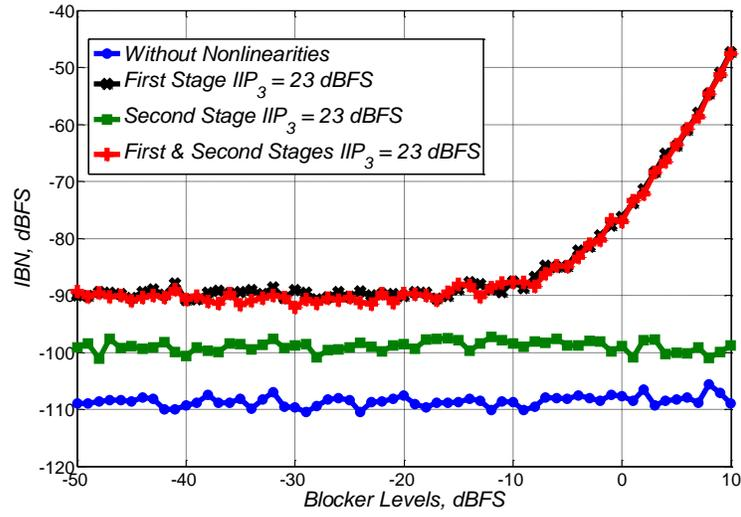
**Fig. 7.6. IBN sensitivity to OOB blocker level due to noise folding, OOB blocker tone at 5.6 MHz,  $A_{SIG} = -65$  dBFS,  $f_{SIG} = 31$  KHz.**
