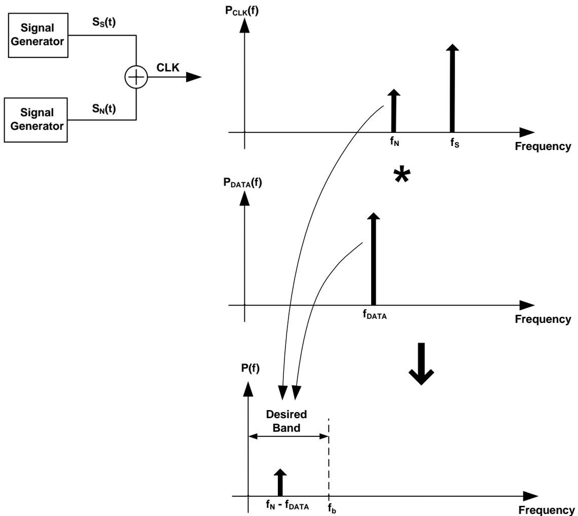
**Fig. 6.8. Testing procedure based on noise tone folding due to periodic jitter in clock.**
