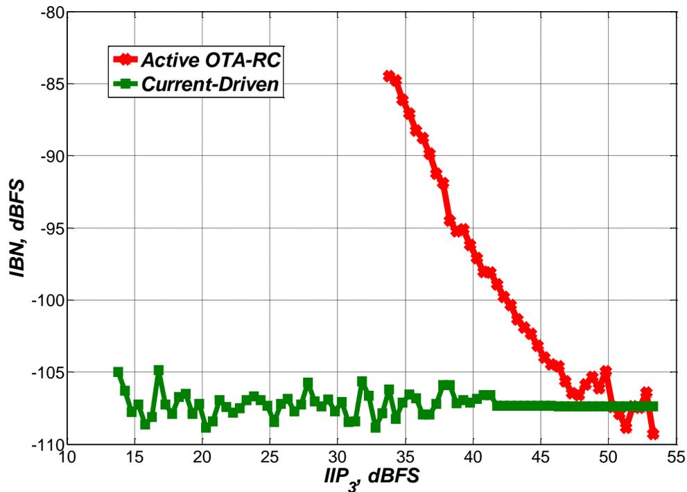
**Fig. 7.10. Sensitivity of total IBN to  $IIP_3$  of the first integrator stage in the loop filter for a current-mode integrator and an active-RC integrator. 6 dBFS OOB blocker tone at 5.6 MHz,  $A_{SIG} = -65$  dBFS,  $f_{SIG} = 31$  KHz.**
