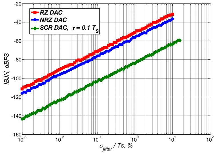
**Fig. 2.20. IBJN plots for the  $\Delta\Sigma$  modulator in Fig. 18 using different DAC types.**
