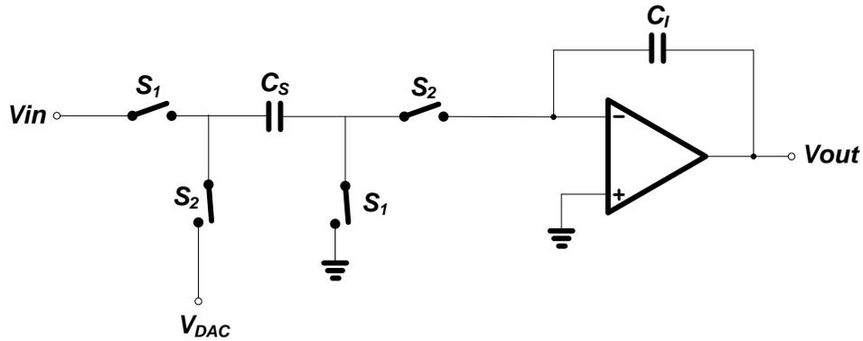
**Fig. 2.12. Non-inverting switched-capacitor discrete-time integrator.**
