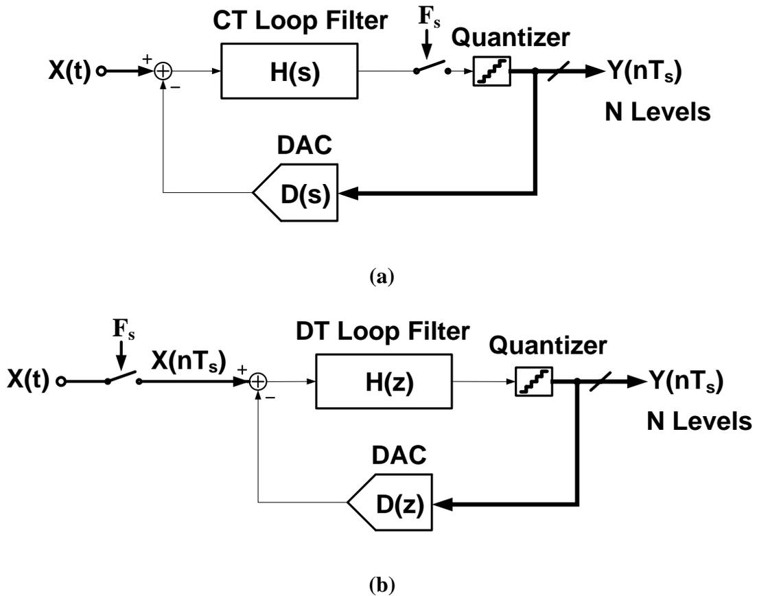
**Fig. 2.10.  $\Delta\Sigma$  Modulators. (a) Continuous-Time. (b) Discrete-Time.**
