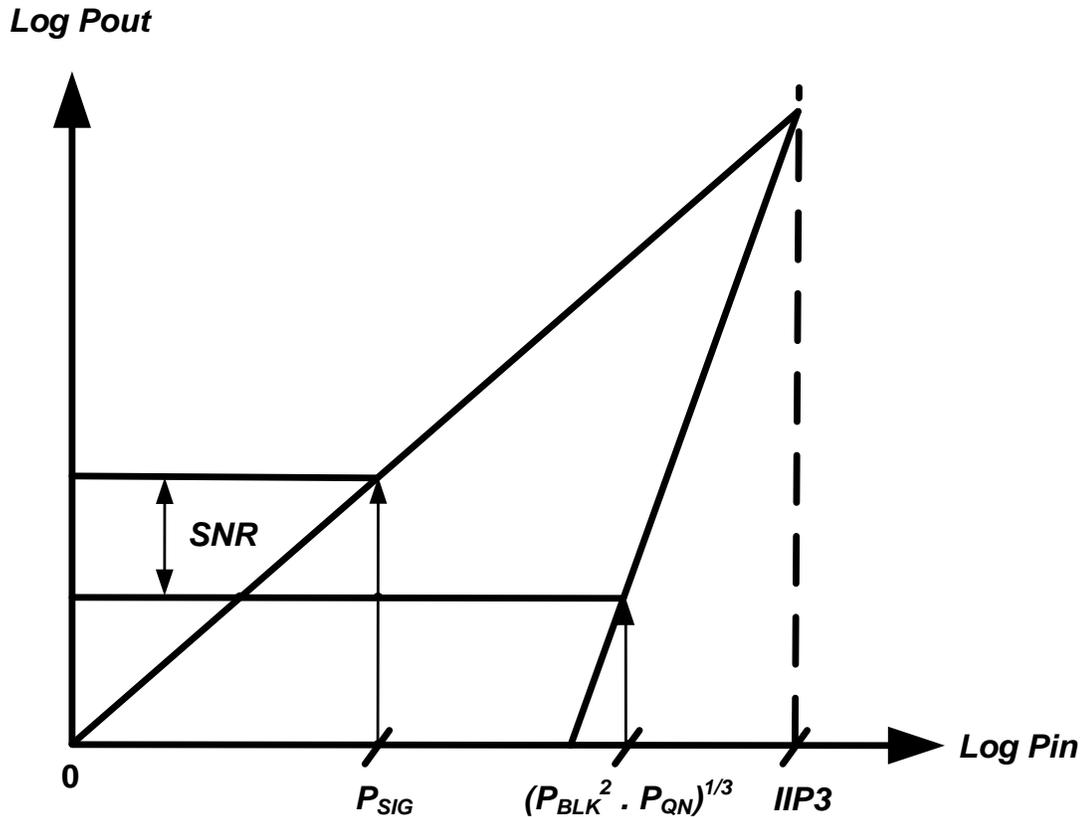
**Fig. 7.3. Derivation of loop filter  $IIP3$  in presence of OOB blockers according to noise folding.**
