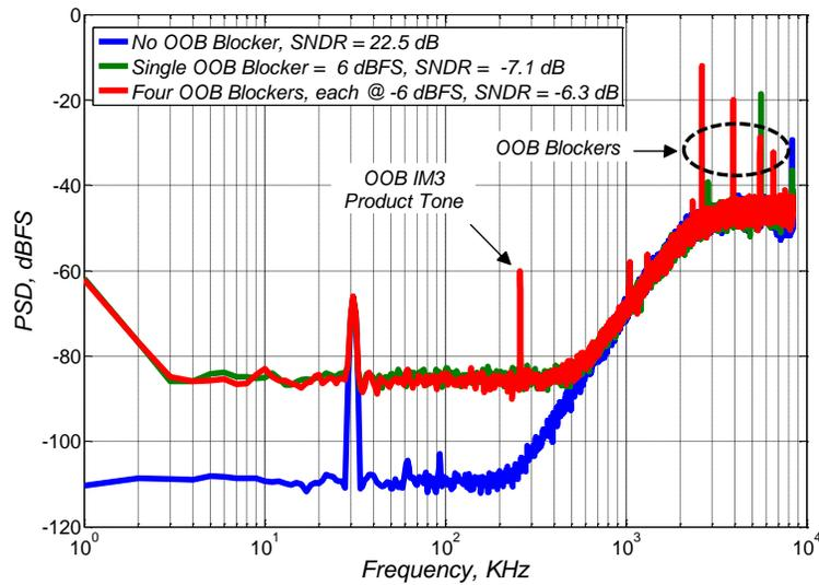
**Fig. 7.7. Power spectra at the output of a third-order CT modulator in presence of single OOB blocker tone,  $f_{BLK} = 5.8$  MHz and four OOB blocker tones,  $f_{BLK1} = 2.63$  MHz,  $f_{BLK2} = 3.94$  MHz,  $f_{BLK3} = 5.52$  MHz,  $f_{BLK4} = 6.57$  MHz,  $A_{SIG} = -65$  dBFS,  $f_{SIG} = 31$  KHz, first stage  $IIP_3 = 23$  dBFS.**
