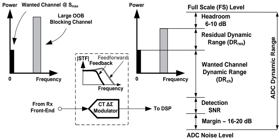
Fig. 3.8. ADC dynamic-range budgeting in presence of blockers.
