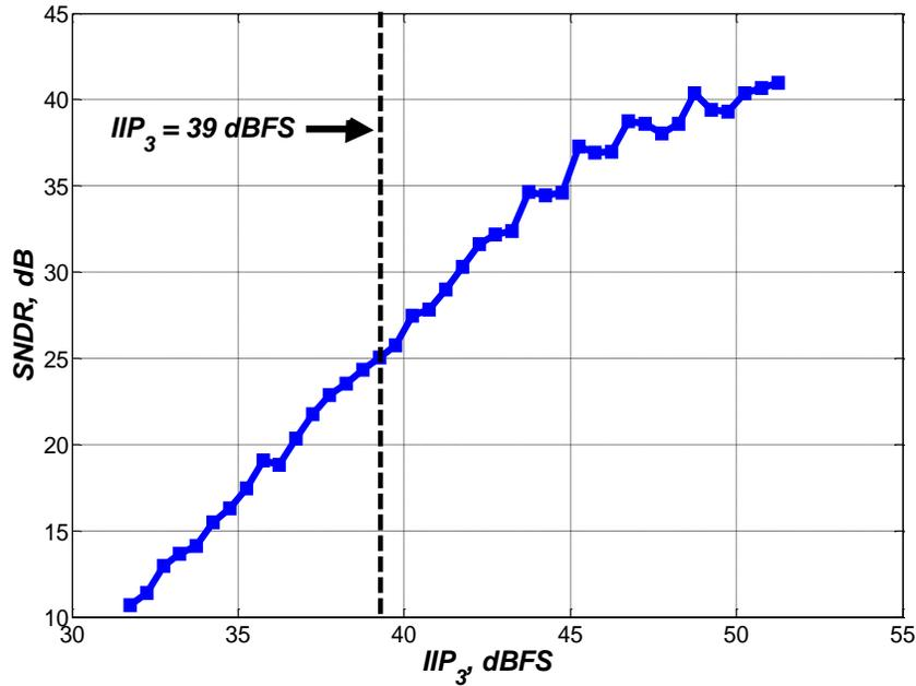
**Fig. 7.8.  $IIP_3$  requirement on the loop filter. 6 dBFS OOB blocker tone at 5.6 MHz,  $A_{SIG} = -65$  dBFS,  $f_{SIG} = 31$  KHz.**
