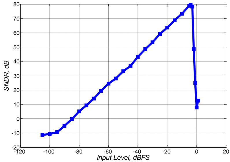
**Fig. 2.17. Dynamic-range of the adopted  $\Delta\Sigma$  modulator.**
