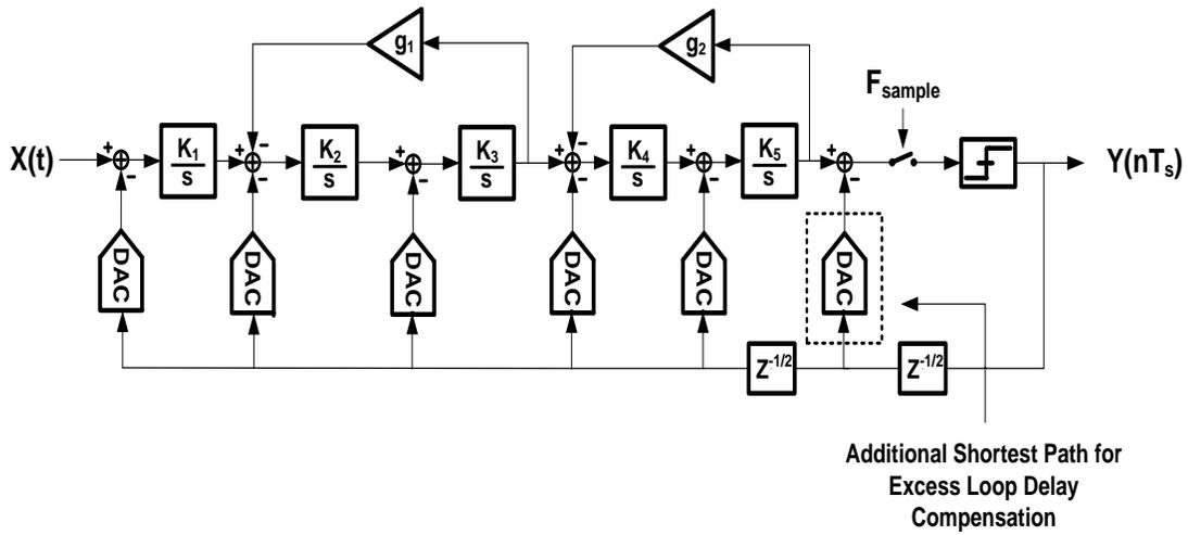
**Fig. 4.1.** Fifth-order continuous-time  $\Delta\Sigma$  modulator in CRFB structure.
