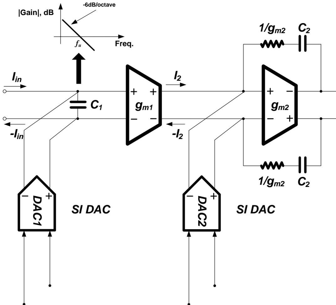
**Fig. 7.9. First two integrator stages in a CT loop filter with a current-mode input integrator stage.**
