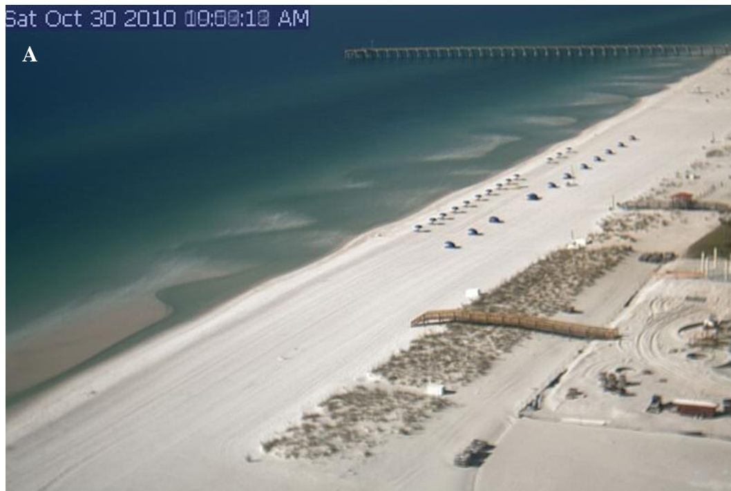
Fig. 1.3. A time-lapse image taken from camera mounted on top of hotel overlooking Casino Beach shows (A) transverse bar and rip morphology on October 30 th , 2010 and (B) a rhythmic bar-beach morphology on September 14 th , 2010.
