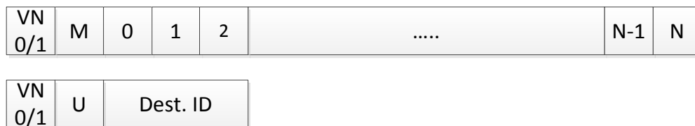
Figure 17. Proposed header format. 3 rd bit is used to differentiate a unicast packet with multicast packet.
