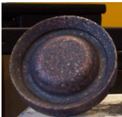
Fig. 4.8.: The copper base fits the bottom of the can and provides uniform heat to the reactor
