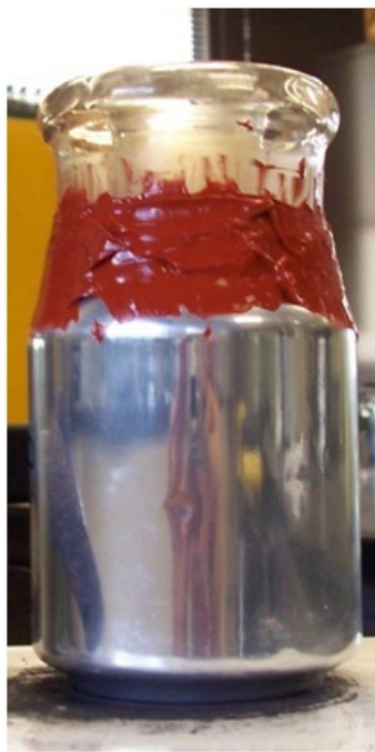
Fig. 4.4.: Reactor elements: glass insert, Al can, and silicon gasket maker
