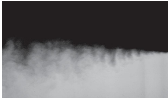
Figure 2.7. Image of test section from gas channel with Atwood number 0.6.
