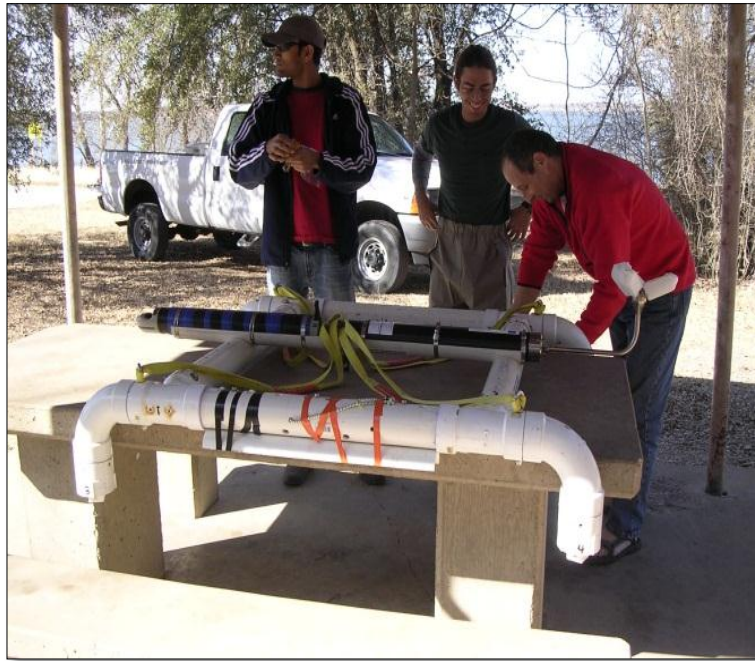
Fig 2.2. ADCP & ADV on the Bottom Mount (Photograph courtesy Dr. Ayal Anis).
