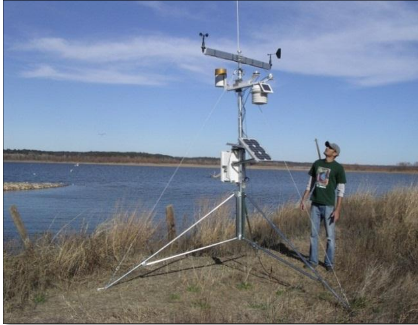
Fig 2.8. Station B Meteorological Measurement Tripod (Photograph courtesy Dr. Ayal Anis).
