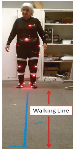
Fig. 2.3.: Straight line human walking experiment with LED sensors placed on various sections of the human subject.
