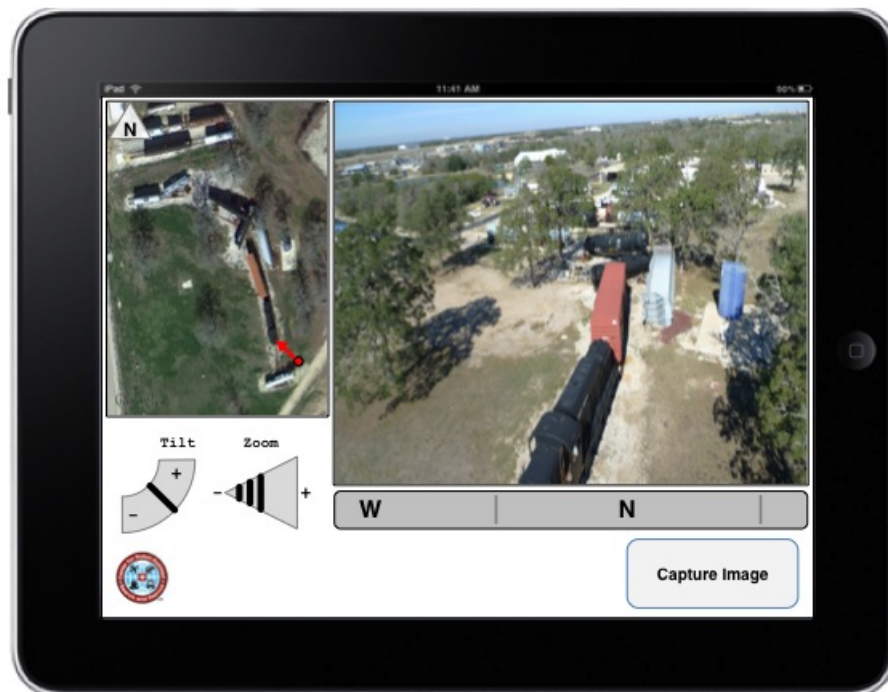
Fig. 5.3. Refinements of the Role-Specific Mission Specialist Interface Informed by the Exploratory Study. A Captured Image of the Simulated Train Derailment is Shown. The Mission Specialist Swipes (Up and Down) and Pinches (In and Out) Directly on the Video Display to Control the Payload Camera for Tilt (Up and Down) and Zoom (Out and In). Images are Captured by Pressing the Capture Image Button. Additionally Added are Zoom and Tilt Indicators, an Overview Map, Position of the Robot, and a Digital Compass (Courtesy of Center for Robot-Assisted Search and Rescue).
