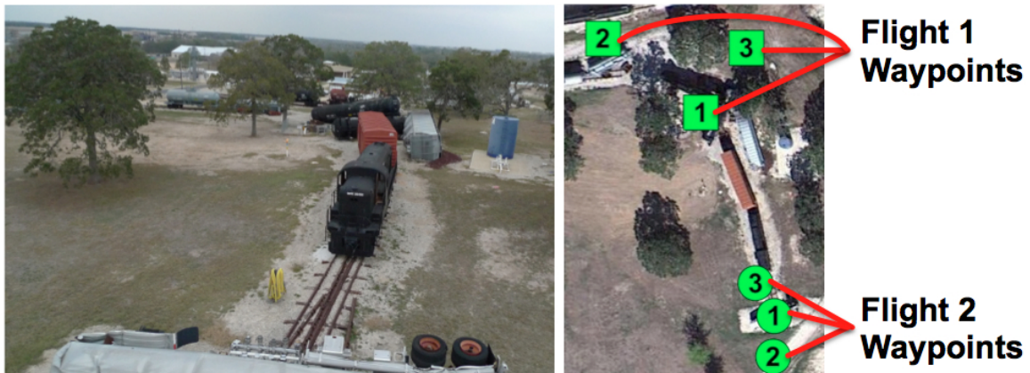
Fig. 6.1. Frontal and Overhead Map Views of the Simulated Train Derailment at Disaster City® with the Three Waypoints Shown for Each Mission Trial. Mission Trial 1 Waypoints are Shown as Circles and Mission Trial 2 Waypoints are Shown as Squares. The Numbers Indicate the Three Waypoints in the Ascending Order They Were Visited (Courtesy of Center for Robot-Assisted Search and Rescue).
