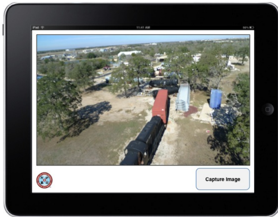
Fig. 5.1. Initial Implementation of the Mission Specialist Interface on an Apple® iPad. A Captured Image of the Simulated Train Derailment is Shown. The Mission Specialist Swipes (Up and Down) and Pinches (In and Out) Directly on the Video Display to Control the Payload Camera for Tilt (Up and Down) and Zoom (Out and In). Images are Captured by Pressing the Capture Image Button (Courtesy of Center for Robot-Assisted Search and Rescue).
