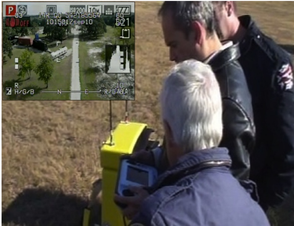
Fig. 1.1. A Micro UAS Mission Specialist (far right) Passively Shares an AirRobot® AR-100B Payload Camera Display with the Pilot (center). The Display (upper left) Contains Numerous Visual Indicators Such as Battery Voltage, Flight Time, Distance from Home, etc. that are Important to the Pilot but not the Mission Specialist (Courtesy of Center for Robot-Assisted Search and Rescue).
