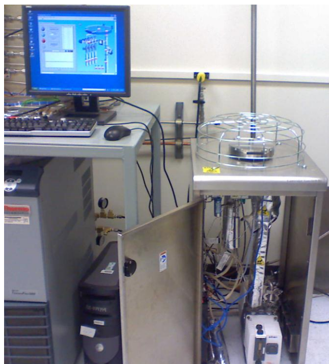
Fig. 12. Image of the Cambridge NanoTech Savannah Atomic Layer Deposition Tool, installed by the author.
