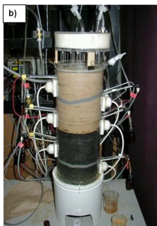
Figure 6.5: Schematic of a) the layered and lensed columns with instrumentation, b) the experimental setup of the layered sand-over-loam column, and c) the experimental setup of the lensed column.
