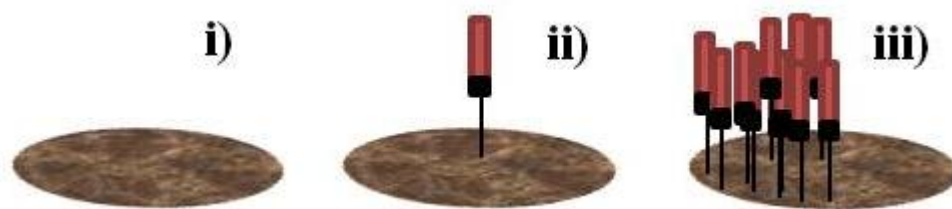
Figure 2.3: Experimental designs: (i) homogeneous soil, (ii) central macropore, and (iii) multiple macropore columns.
