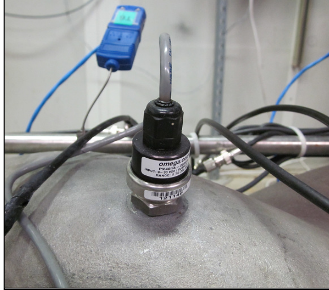
Figure 4.15 : Location of a pressure and temperature sensor.
