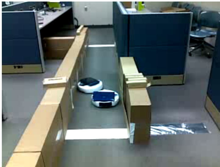
Fig. 2. Physical robots traversing a narrow corridor at the same time results in spatial interference.
