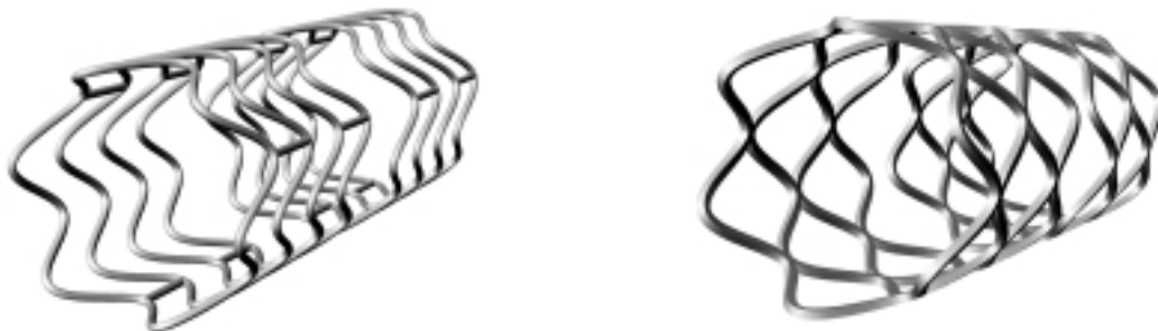
Figure 1. Stent models based on Guidant Multilink and Palmaz-Schatz PS 153 designs.
