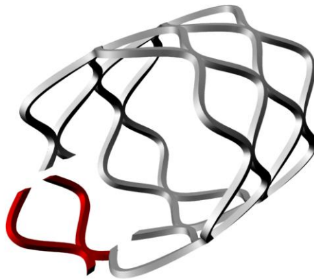
Figure 3. Partial model of stent cut from a full stent (slotted tube design)
