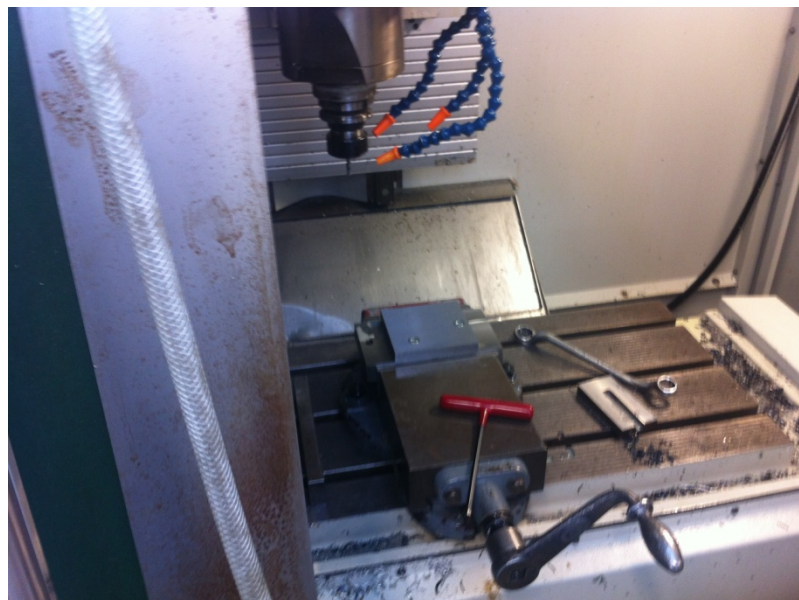
Fig. C.2 Clamping the test piece into the machine
