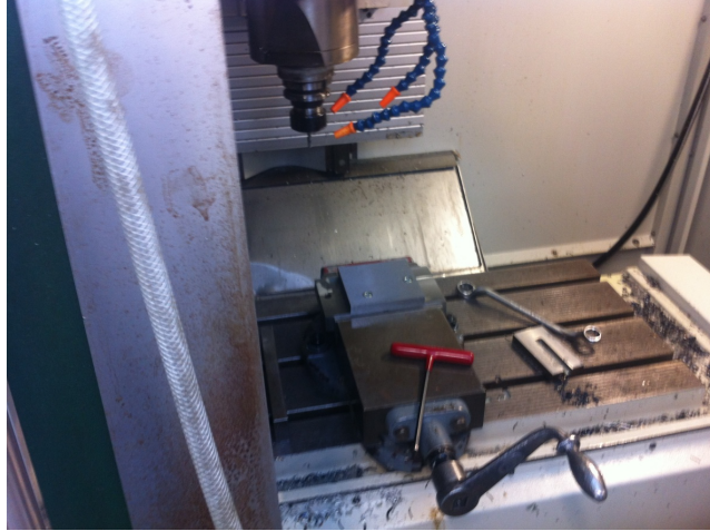
Fig. 4.5 Steel block clamped into the 3 axis milling machine
