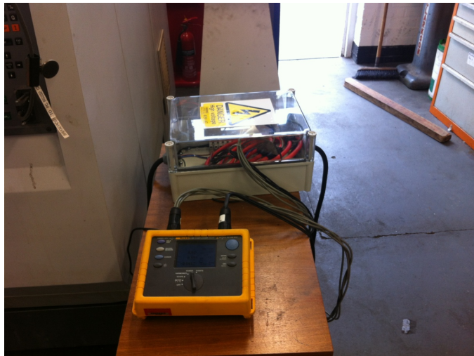
Fig. 4.6 The power logger connected to the 3 phases motor
