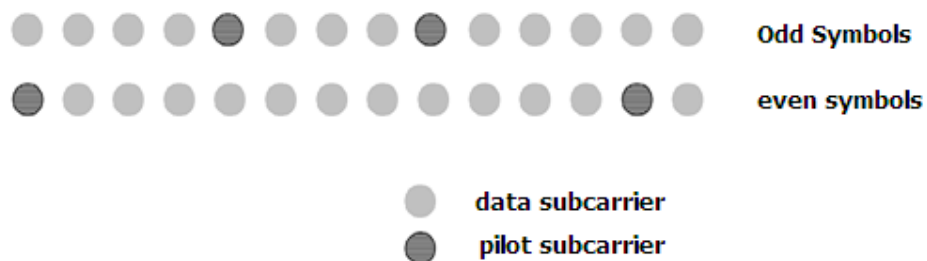
Figure 7: DL-PUSC Cluster Structure [1]
