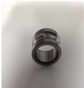
Figure 4. Inner race fault.
