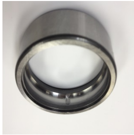
Figure 3. Outer race fault.
