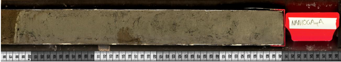
Figure 4.3: Characteristic core image of sediment Unit A from Nanerersarpik Lake. Unit A consists of dense, minerogenic clayey silt with high magnetic susceptibility.
