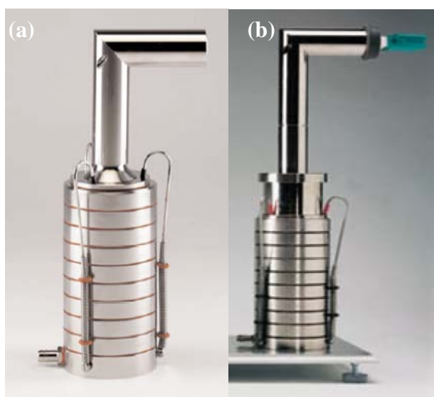
Figure 2.31 (a) Anderson Cascade Impactor set for MDI. (b) Anderson Cascade Impactor set for DPI (Reproduced from Copley, 2008).
