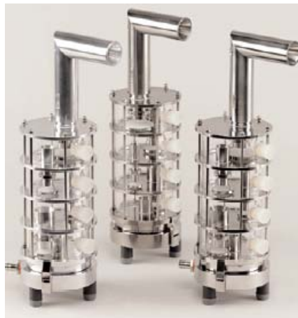
Figure 2.30 Multistage Liquid Impinger (Reproduced from Copley, 2008).
