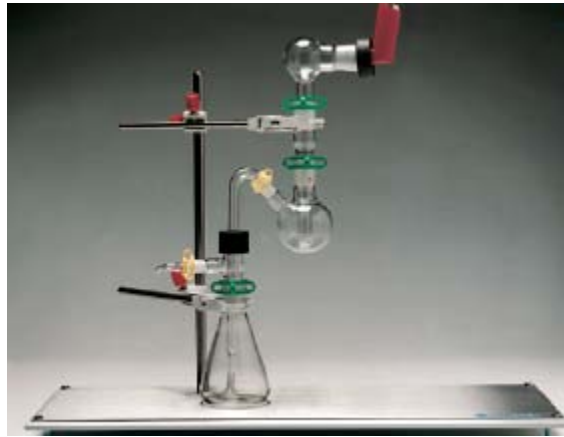
Figure 2.29 The Twin Stage Impinger (Reproduced from Copley, 2008).
