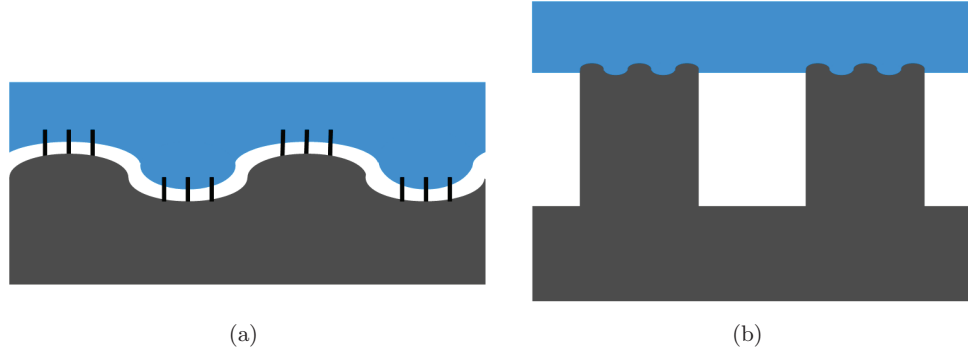
Figure 3.3. Schematics of two different scenarios of partial Wenzel state: (a) type-I: only primary features are penetrated, and (b) type-II: only secondary features are penetrated.
