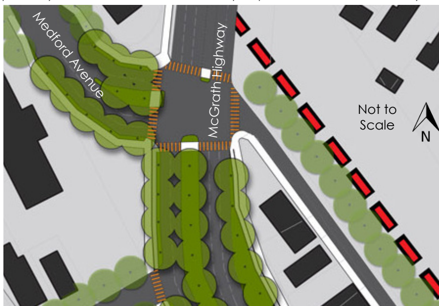
The McGrath and Medford Street: Reducing the lane widths allows for a wider infiltration area to be created on the east side of the highway. This will serve as the beginning of a park system that carries throughout the remaining corridor and includes connections to the Community Path.
