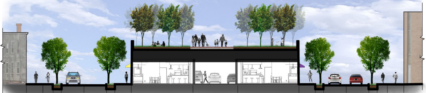
The McGrath Highway Proposed Section A-A': This proposed section shows how the varies elements work together and how a livable street can be created. Shops are located beneath the elevated park and infiltration areas as well as pedestrian and bicycle networks are incorporated.
