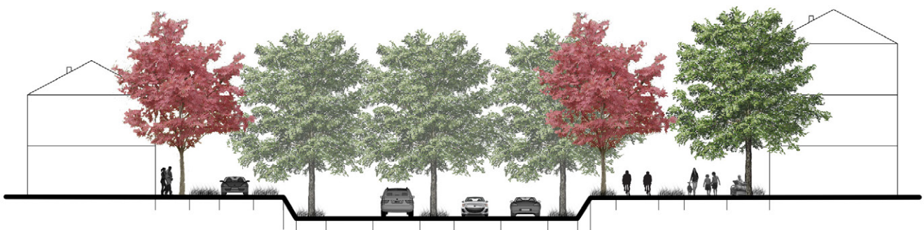
Proposed section at Everett Street: The McGrath Highway travel lanes have been narrowed to 12'. A Boulevard has been depressed 6' with tree plantings and infiltration basins to aid in air and water quality, as well as to buffer highway noise. A Linear park with pedestrian and bike paths shown to the east. Shared street shown to the left with infiltration basins and narrowed travel lane.
