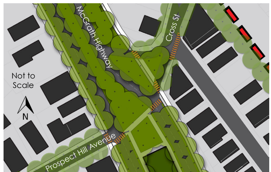
The McGrath Highway, Prospect Hill Avenue, and Cross Street Proposed Plan: The redesigned intersection allows for pedestrians to cross and enter East Somerville. The design also increases the tree canopy and allows the elevated park to return to a boulevards street.
