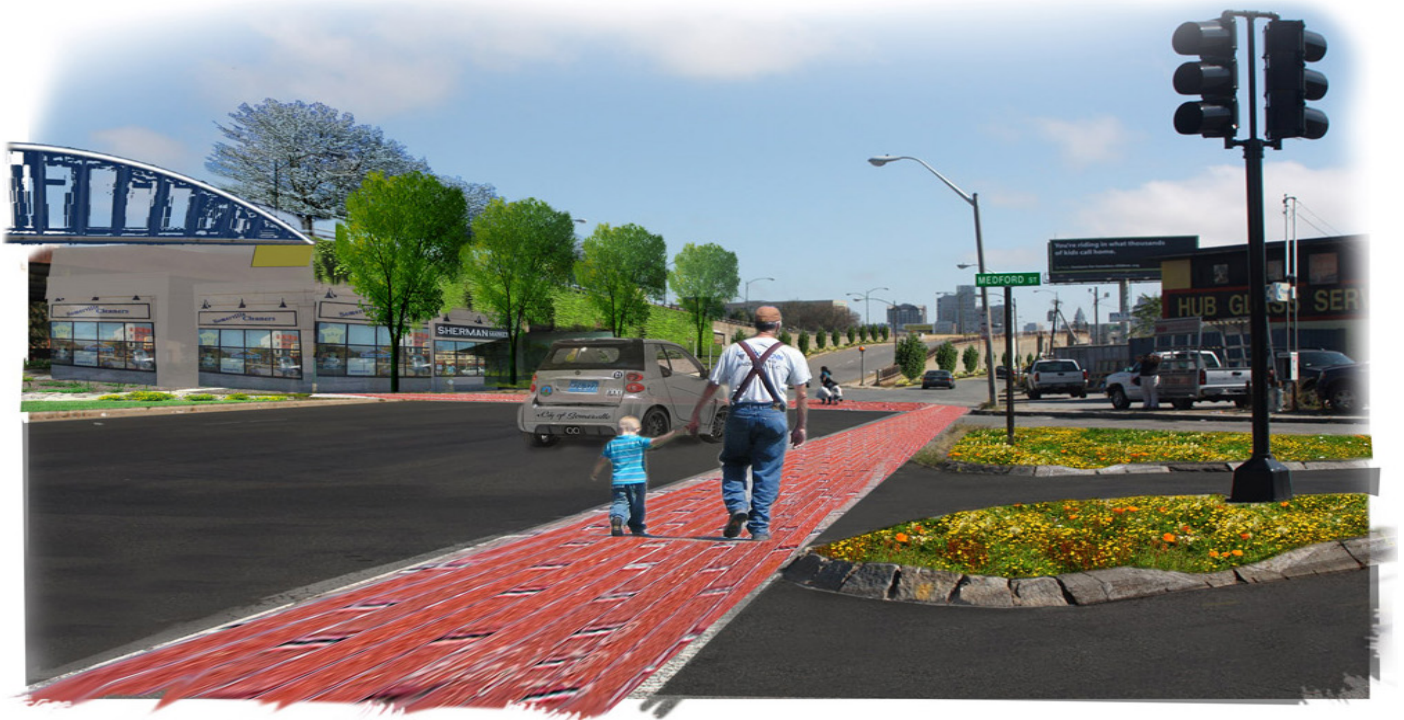
The McGrath Highway and Somerville Avenue Proposed Photomontage: The elevated portion of McGrath is converted into an elevated park with commercial areas below. A pedestrian bridge and increased pedestrian elements are incorporated to create a much safer crossing. Increased tree canopy and infiltration areas help reduce the amount of stormwater entering the CSOs.
