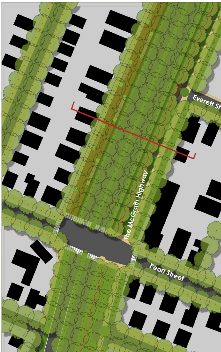
Site plan: Mid-McGrath corridor, showing linear park to the east and shared street to the west of McGrath.
