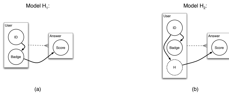
Figure 3.10: Alternative models that explain the marginal dependence between Stack Overflow badge awards on user and scores of their answers. In (a), badge awards have a direct influence on answer score; in (b), the perceived dependence is due to instance dependence bias brought on by a hidden factor H . The two models can be differentiated by performing a conditional hypothesis test on ID and Score conditioned on Badge .
