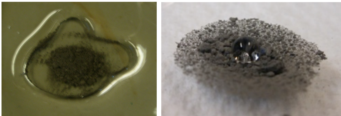
Figure 3.9. Images of nickel powder modified with D 4 -vapor for 72 hours at 150 °C illustrating their hydrophobicity by pushing water away preventing the spreading of water on glass (left) and creating a hydrophobic raft floating on water and supporting a water droplet.
