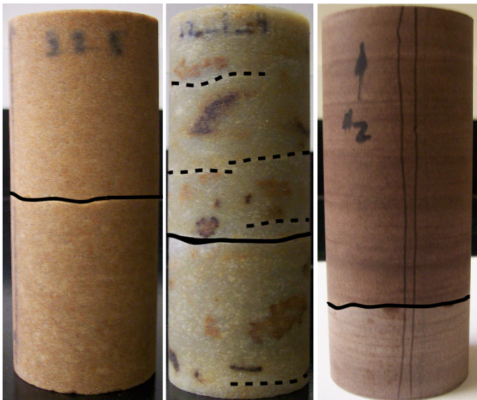
Figure 2.2. Core images after NHF experiments. A) Each core with one primary through going fracture. B) Cores with NHFs outlined in black and non-through going fractures outlined in dashed black lines (French, 2010).
