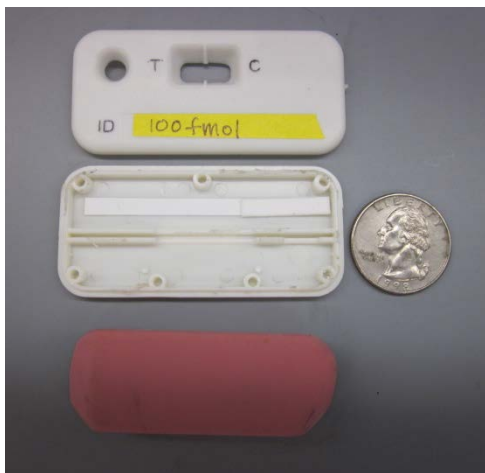
Figure 3.9- Novel test strip housed in a commercial plastic cassette.
