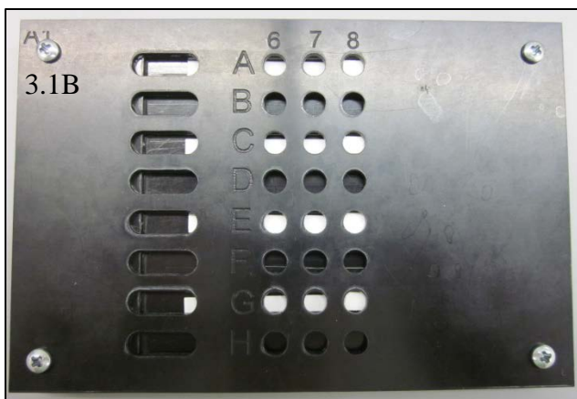
Figure 3.1B- The assembled 96-well plate used to measure fluorescence produced by the ruthenium-doped SiNPs. The lid was placed on top of the tray holding the test strips and was held in place with screws. The exposed areas were read by the Biotek plate reader much like a normal 96-well plate.
