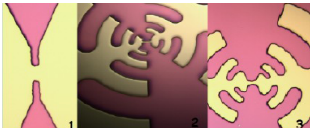
Figure 3.1: Results of development after UV lithography. Purple areas indicate soon to be metalized areas. Device 1 is termed 9 \mu m Bars, 2 is LPA2 1 and 3 is LPA4.
