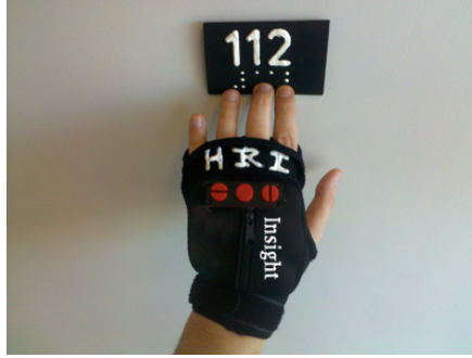
Figure 3.3.RFID Glove (back view) Scanning an R-Tag
