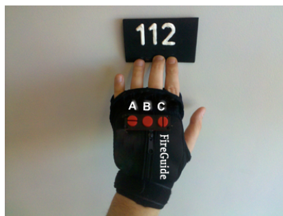
(A).RFID Glove (back view) Scanning an R-Tag
