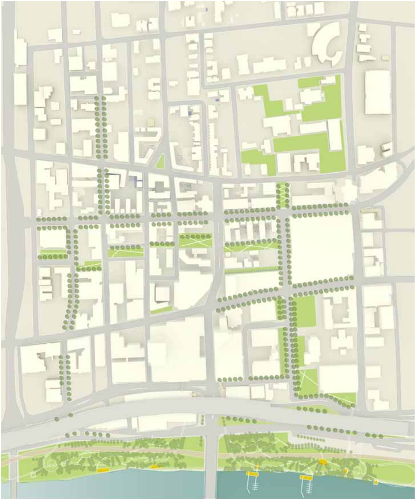
This master plan displays the existing and proposed open spaces linked by the enhanced Court Street axis and the new north - south connection from Mass Mutual to Union Station. Hampden Street is also redesigned to facilitate pedestrian and bicycle circulation.
