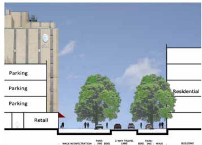
Dwight Street looking north with new residential buildings on the right and the urban supermarket block on the left. The impervious surface in the 70' wide layout of Dwight Street has been reduced by two-thirds.
