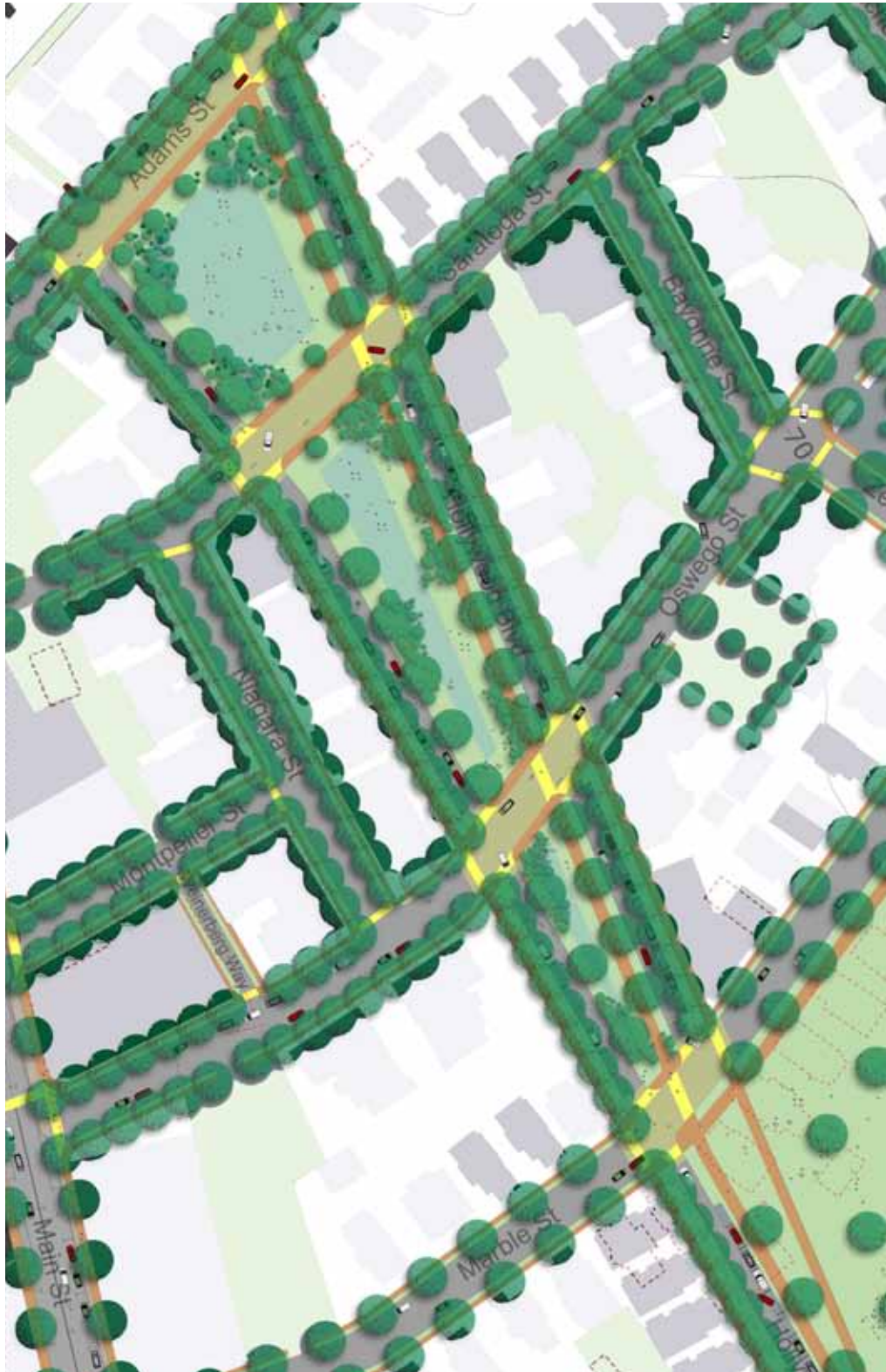
Plan of the Hollywood Mall that connects to Emerson Wight Park in the South. – Existing buildings are in light gray. Proposed Buildings are in dark grey. Demolished buildings are transparent with a dashed red border. Pedestrian crosswalks are yellow; Raised pedestrian crosswalks are located along Hollywood Boulevard at every cross street. Pedestrian pathways are show in orange. Parking lots and streets are in light gray.
