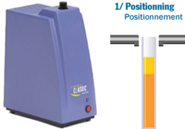
Figure 3.3 Photograph of Turbiscan and Schematic scan mode. The Turbiscan MA 2000 reads transmission and backscattering data every 40 \mu m while reading head move along the cell height [121].
