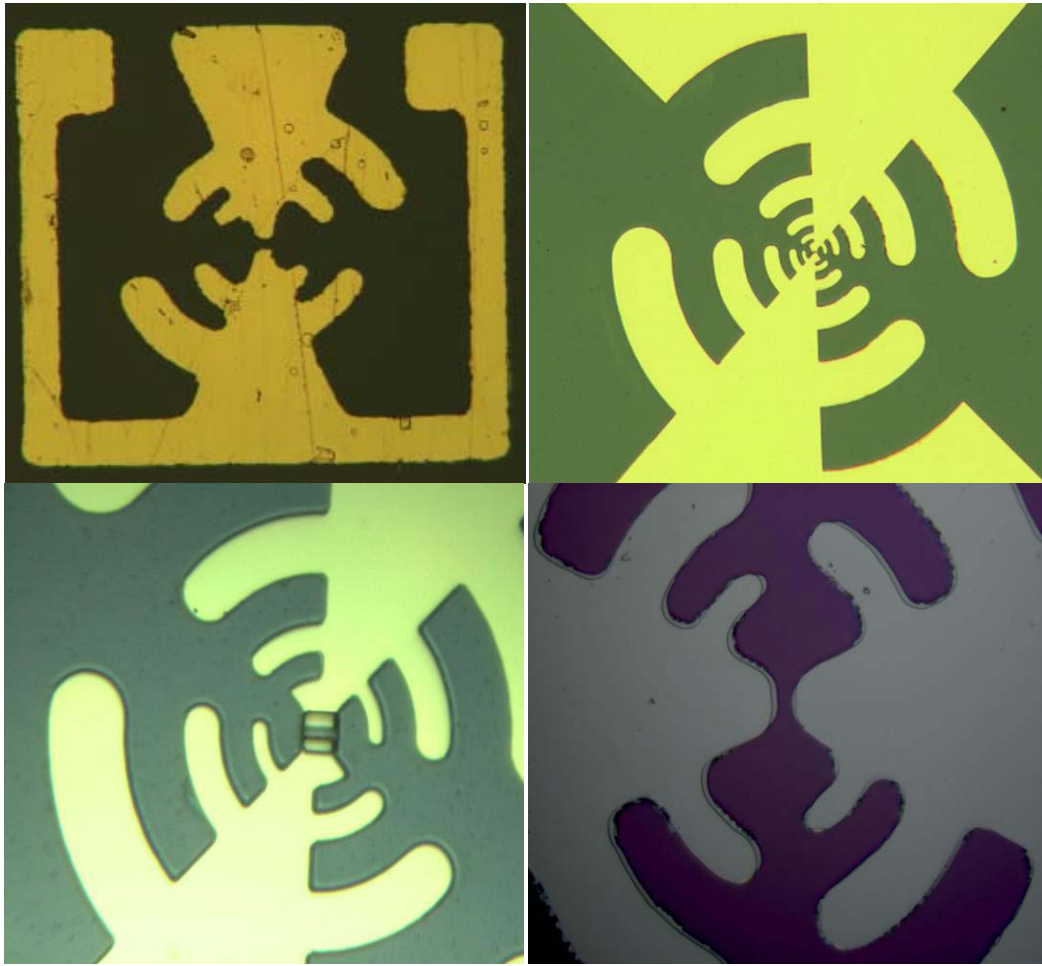
Figure 2.2 Optical pictures of the four generations of LPA used in this work: LPA1 (Top Left), LPA2 (Top Right), LPA3 (Bottom Left), and LPA4 (Bottom Right).
