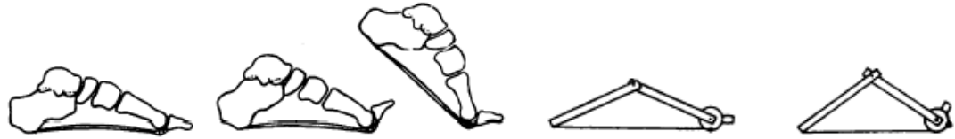
Figure 8. The windlass mechanism (Hicks, 1954).
