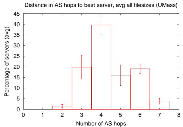
Figure 14. Distribution of the distance to best servers in AS hops for UMass; avg. of all file sizes and all 193 servers.
