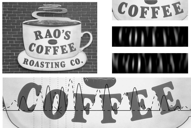
Figure 3: Grating operator on text. UPPER LEFT: Input image. UPPER RIGHT: Center-on and center-off simple filter responses ( \theta = 0 ). BOTTOM: Slice of simple filter responses and receptive regions for a marked point.
