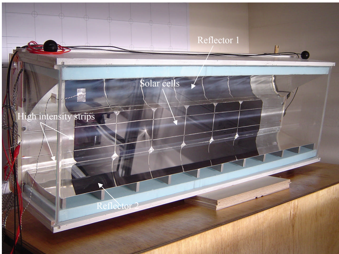
Figure 5.32 Experimental characterization of an ACPPVC-55 system at a solar incidence angle of 10^\circ (from the horizontal) using the developed collimated solar simulator detailed in Chapter 4
