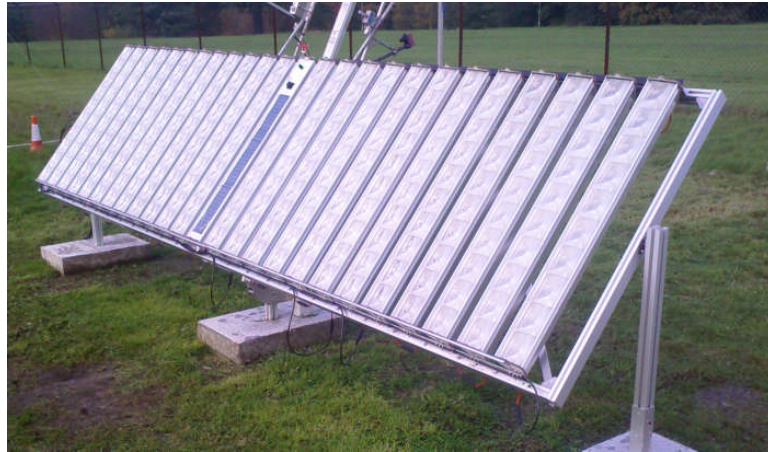
Figure 6.1 A photograph of the Fresnel Lens PV Concentrator (FPVC) systems developed by 'Whitfiled Solar' Company
