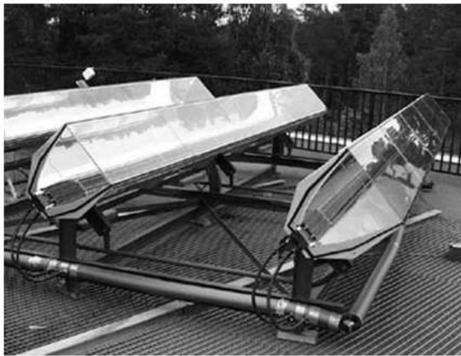
Figure 1.35 Water cooled PV-thermal hybrid system with a low concentrating aluminium Compound Parabolic Concentrator (Brogren et al, 2001)
