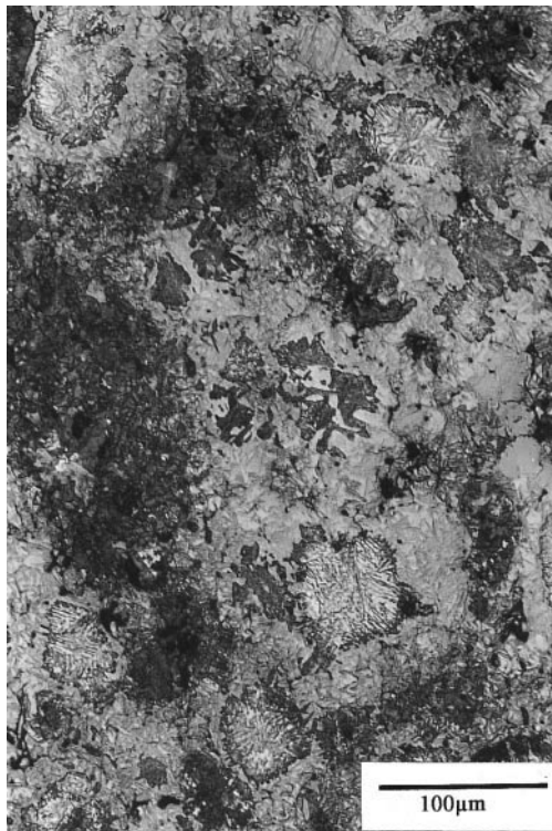
3 Optical micrograph of Fe-0.5Mo-3Mn-0.8C sintered at 1120°C with dewpoint of -60°C: improved diffusion and much smaller presence of oxides compared with Fig. 2 illustrate the effect of improving the dewpoint from -35 to -60°C
