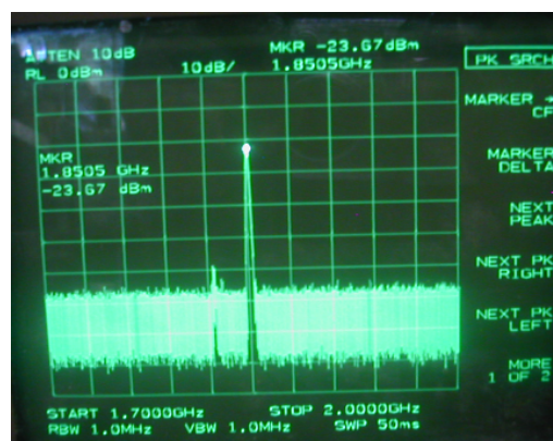
Figure 7: The output of the back to back baluns when the switch mode is on.
