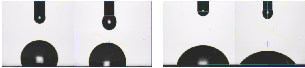
Figure 2: Contact Angles of Paper1 ( 117^{\circ} to 110^{\circ} after 30s) and Polyester2 ( 77^{\circ} to 46^{\circ} after 30s).
