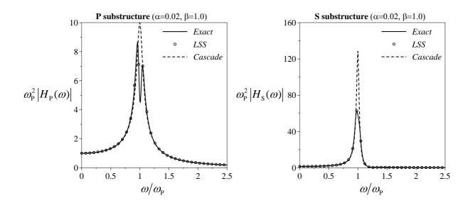
Dimensionless absolute value of the Frequency Response Functions of the 2-DoF combined P-S system with mass ratio  $\alpha = 0.02$  and tuning parameter  $\beta = 1.0$ : P oscillator (left); S oscillator (right).
