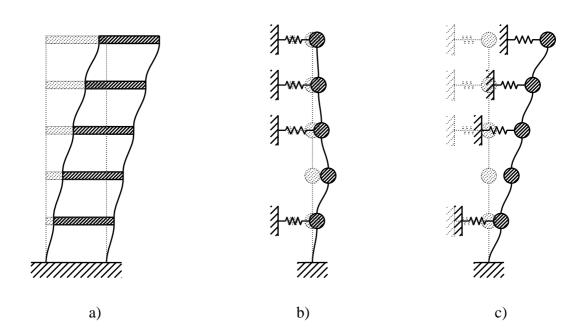
Modal shapes of the P structural system (a) and of the base-fixed S attachment (b); deformed shape of the S attachment induced by the modal shape of the P structural system (c).
