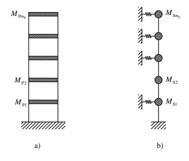
Base-fixed substructures: P structural system (a); S attachment (b).
