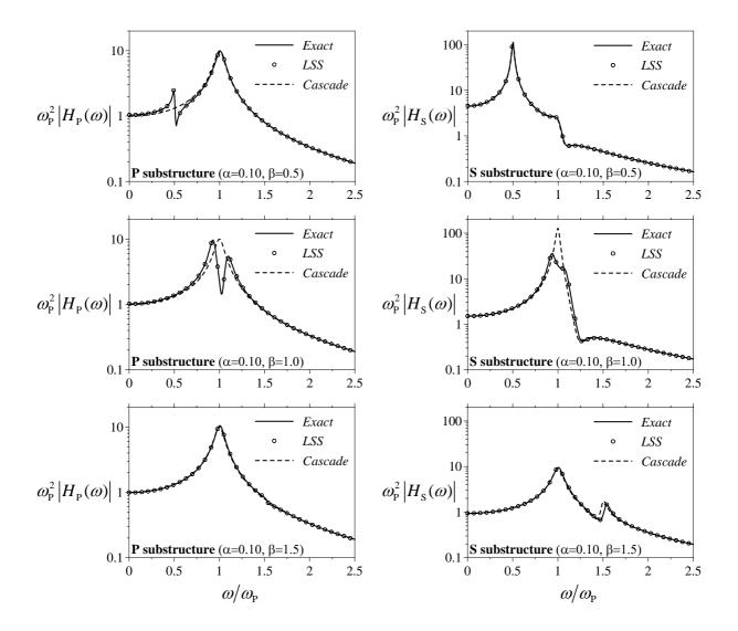
Dimensionless absolute value of the Frequency Response Functions of the 2-DoF combined P-S system with mass ratio  $\alpha = 0.10$  and tuning parameters  $\beta = 0.5$ , 1.0 and 1.5 (log-linear plots): P oscillator (left); S oscillator (right).
