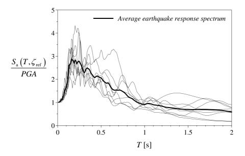
Normalized response spectra for the recorded accelerograms listed in Table 2 (thin lines) and average earthquake response spectrum (thick line).
