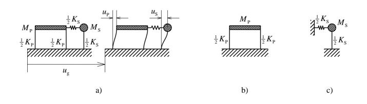
2-DoF combined P-S system (a); P oscillator (b); S oscillator (c).
