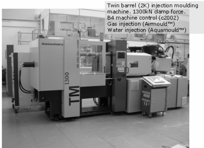
Figure 5: Battenfeld injection moulding machine with separate gas / water injection controller shown in the foreground. The water injection reservoir is shown behind the machine.
