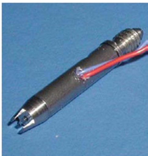
Figure 2-7. A single jet dispensing device (MJ-A style) manufactured by MicroFab Technologies. (www.microfab.com)
