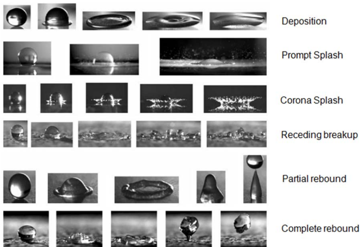
Figure 2-17. A variety of morphologies of liquid drop impact on to a dry surface. (Rioboo et al. 2001)
