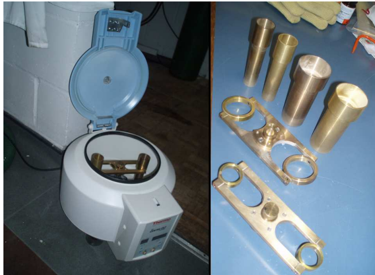
Figure 3.5: The centrifuge used to spin our samples (left) and the two sets of brass moving pieces used for smaller and larger growths (right). Penny pieces were used to balance growths and quartz wool was used to cushion them during the spin. Samples were placed in the centrifuge from the furnace, and the centrifuge switched on. Once it had got to about 3000 rpm, which typically took 7 seconds, the centrifuge was turned off and samples left to cool.
