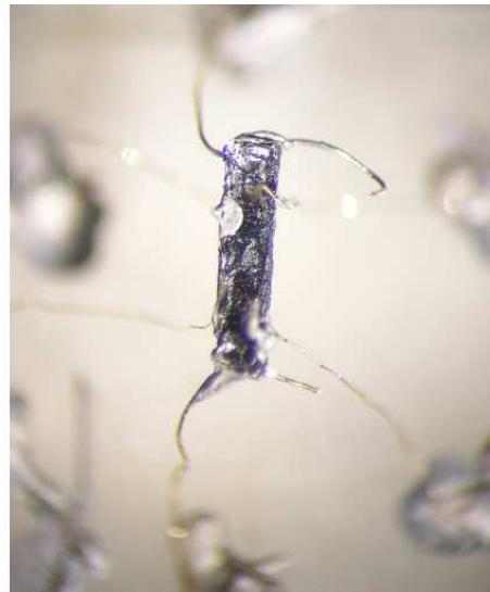
Figure 6.2: A schematic diagram of the setup to measure hall resistance. To allow a uniform current flow, a bar-like morphology is preferred. Here, length > 5 \times width. Two current leads of 50\mu\text{m} diameter are connected at either end, and two pairs of voltage leads of 25\mu\text{m} diameter are connected on opposite sides of the bar. The configuration can be checked by first measuring V vs. T using the terminals on the same side of the bar, the results should be close to each other if contacts are well spaced. Then, measuring V vs. T across the crystal with a current flowing in a perpendicular B -field allows measurement of the Hall effect. The photo above shows a sample I mounted. Ideally contacts will cover the whole thickness of the crystal to avoid any component of out-of-plane resistivity, but will not spill onto the crystal surface.
