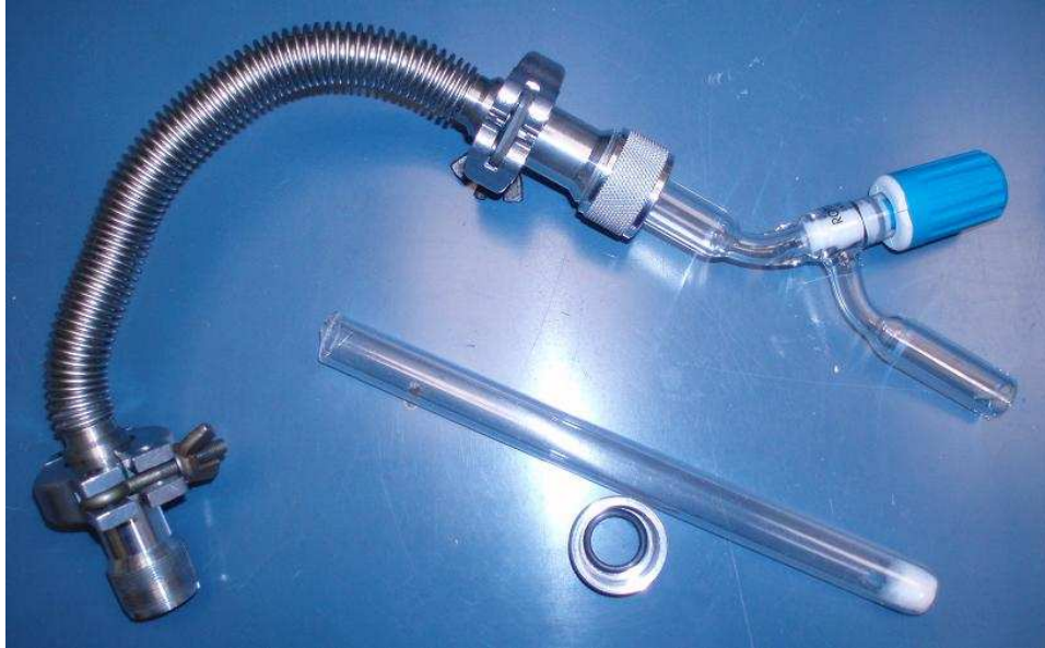
Figure 3.4: Custom-made glassware and brassware for sealing under inert atmosphere. The blue plastic piece is the 'rotaflow' valve, attached via a brass demountable o-ring vacuum seal for quartz tubing, with another on the other end
