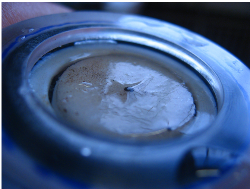
Fig. 6.33 During crushing, the thin plastic membrane may be seen to drape over pellets, resulting in a water-filled void between the sides of the pellet and the membrane.
