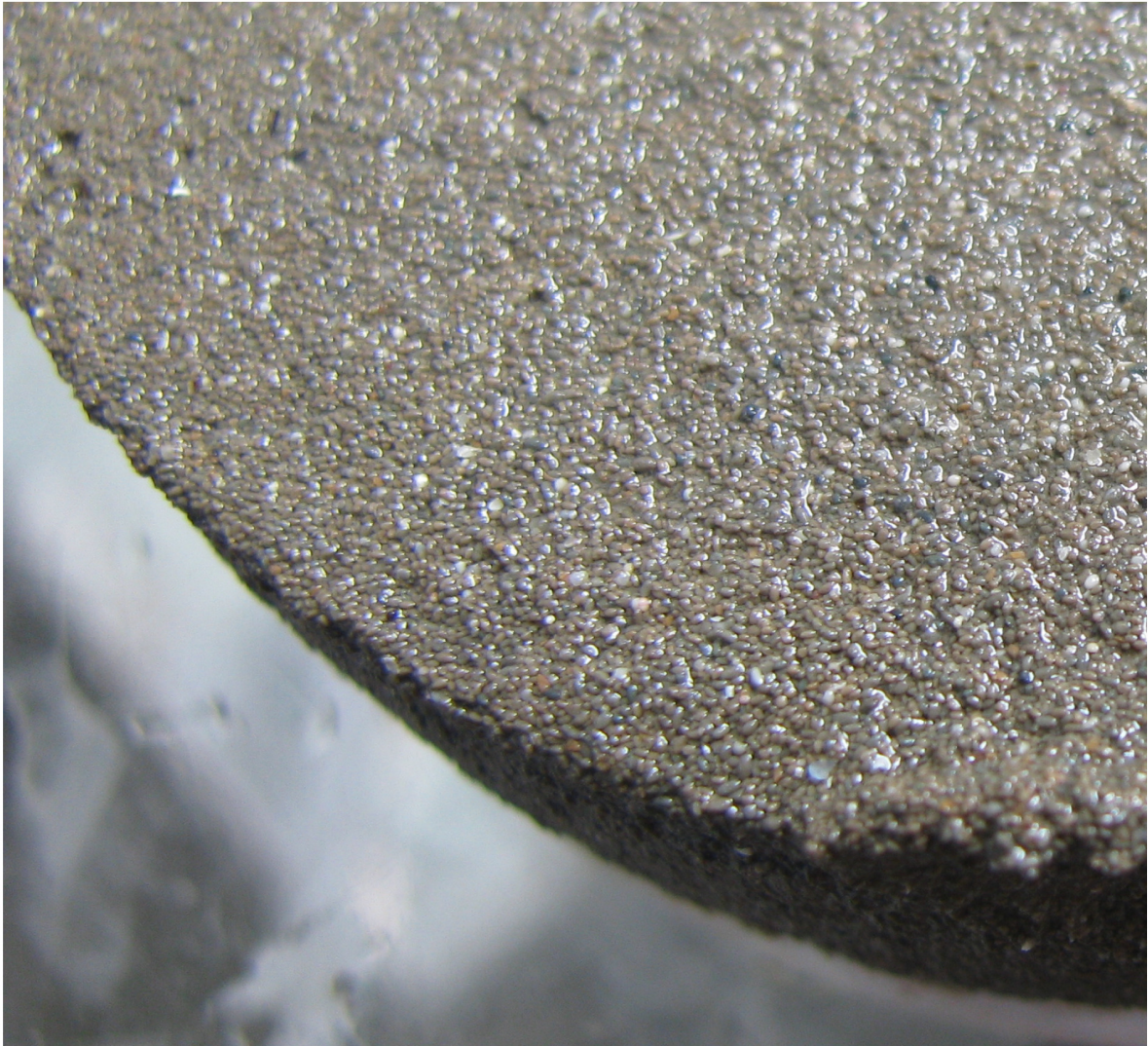
Fig. 6.40 Photograph of intact pellets that were located at the smooth interface after shearing, demonstrating that no crushing had occurred.
