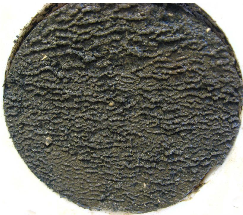
Fig. 6.6 Photograph showing the grainy, undulating texture of a core sample cut with a cheese wire, suggesting the presence of coarser grains.
