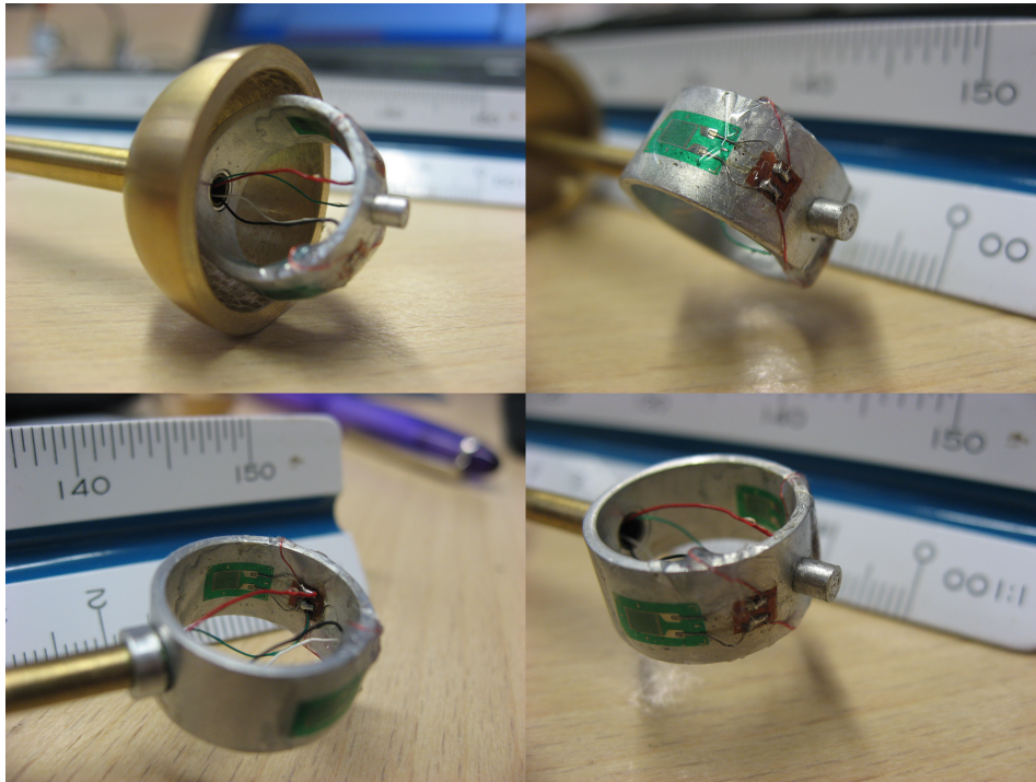
Fig. 3.25 Photographs of the strain-gauged, 1mm thick Dural ring inside the mini ball penetrometer, showing the location of the four strain gauges, and the wires passing through the central push-rod.
