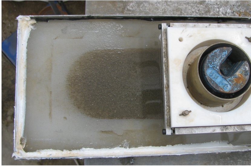
(a) Photograph of smearing due to crushing of pellets observed while shearing on the rough interface.
