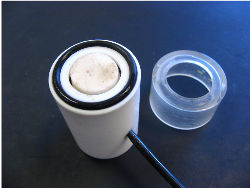
Fig. 6.30 Novel pellet-crushing device used to apply a crushing stress onto pellets by the application of suction to a thin plastic membrane.
