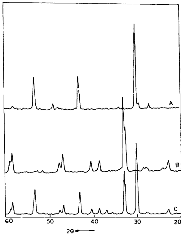
Figure 4.1: Powder diffraction pattern for a) pure \text{Ba}_2\text{YNbO}_6 , b) pure \text{YBa}_2\text{Cu}_3\text{O}_{7-\delta} , c) 1:1 mole mixture of \text{YBa}_2\text{Cu}_3\text{O}_{7-\delta}:\text{Ba}_2\text{YNbO}_6 heated at 950 °C for 15 hr. [4]
